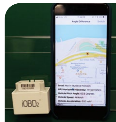
The navigation system uses an ordinary smartphone which is connected to an onboard diagnostic device by Bluetooth.
