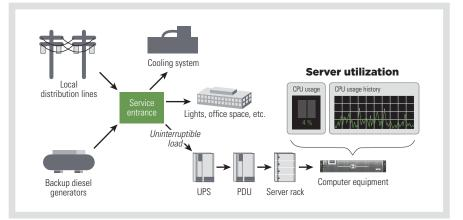
Figure 2. Facilities and IT components that contribute to energy usage
