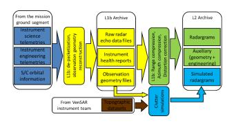
The main steps in L2 processing are azimuth compression (trough SAR processing), range compression and, if needed, correction of ionosphere distortion. Azimuth compression will consist of the sum of a number of echoes, after compensation for their relative delay as the distance of the spacecraft from the target changes along the trajectory. If plasma is present
