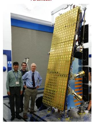
The NovaSAR-S phased array consists of  $3 \times 6$  phase centres (gold panels); VenSAR will comprise an array of  $6 \times 4$  phase centres.
