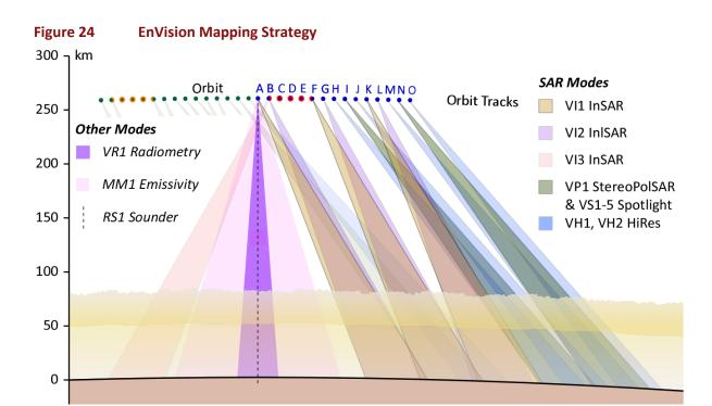
This rather complex figure illustrates the VenSAR mapping sequence for the ~16 orbits in every 24 hours: 4 orbits are reserved for telemetry (open circles); 3 pairs of orbits for InSAR (VI1 and either VI2 or VI3); 2 orbits for StereoPolSAR; and 4 orbits for HiRes and Spotlight. Sounder, Radiometry and VEM data are collected on every mapping orbit; VEM-M and VEM-H on the night side and VEM-U on the day side.
