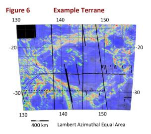
Magellan SAR image with false colour regional slope, showing an average-sized tectonic terrane comprising an undeformed interior (blue) surrounded by relatively diffuse deformation belts (green to red). Notice that these outline neighbouring terranes.
