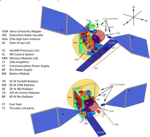
The +z anti-nadir face is free but internally supports the primary bus power distribution subsystem and batteries, and the communications subsystem connected to the +x
