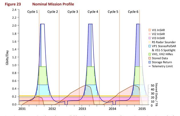
Imaging strategy is adapted to available telemetry rate: towards superior conjunction only the essential InSAR and sounder data are acquired and stored; as the available bandwidth increases towards inferior conjunction, stored data are returned while StereoPolSAR and HiRes data are also acquired.
