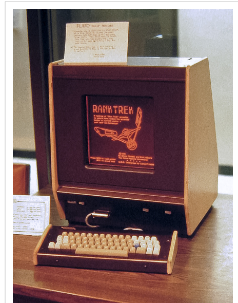
A PLATO V terminal in 1981 displaying RankTrek application, one of the first to combine simultaneous local microprocessor-based computing with remote mainframe computing.
