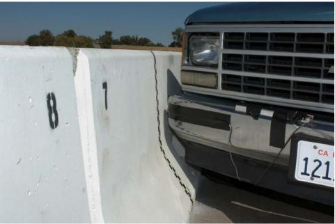
Figure 2-46. Test 674 - Close-up View of Vehicle at Impact Location
