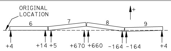
Figure 2-49. Test 674 - Barrier Static Displacements [mm]
