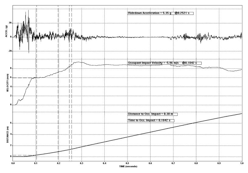
Figure 7-40. Test 676 Vehicle Lateral Acceleration, Velocity, and Distance Vs Time
