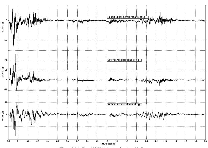
W11: Test 673 - k-rail staking Configuration 2, Longitudinal, Lateral and Vertical Accelerations
