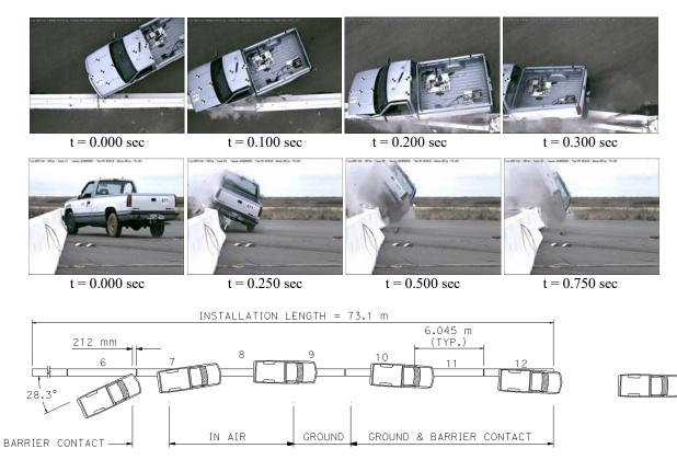
Figure 2-17. Test 671 - Impact sequence and diagram
