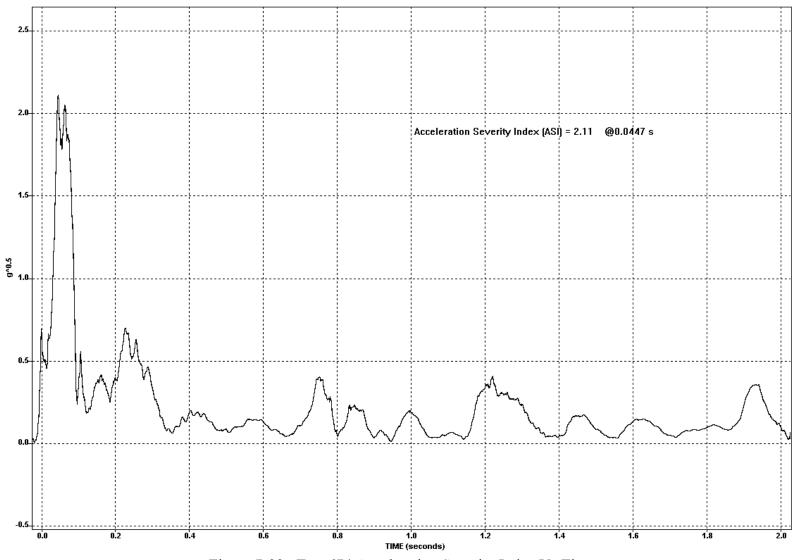
Figure 7-32. Test 674 Acceleration Severity Index Vs Time
