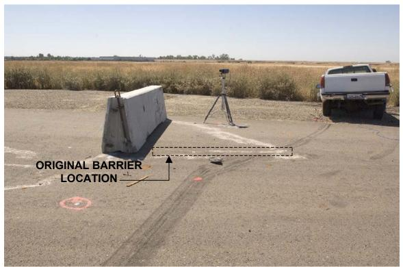
Figure 2-42. Test 673 - Barrier Involved with Secondary Impact
