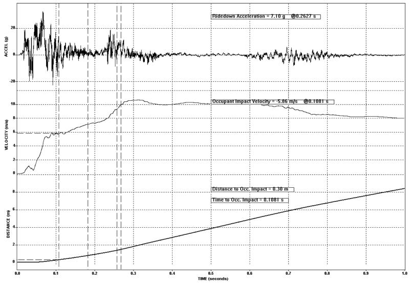
Figure 7-36. Test 675 Vehicle Lateral Acceleration, Velocity, and Distance Vs Time
