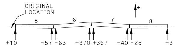
Figure 2-10. Test 671 - Barrier Static Displacements [mm]
