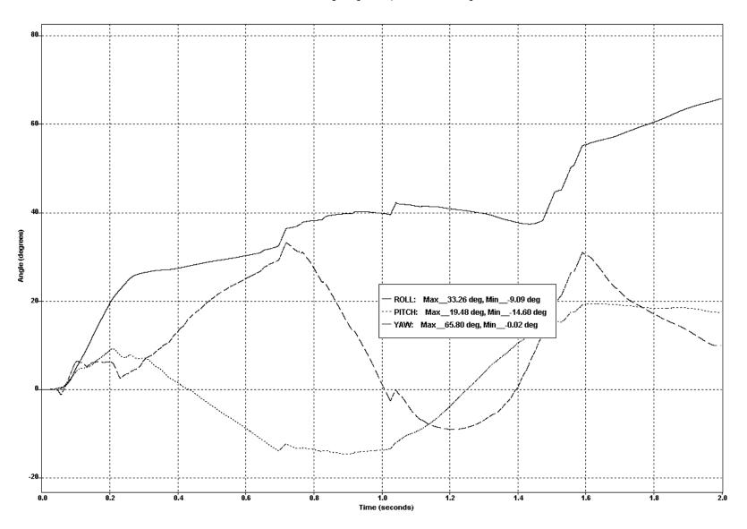
Figure 7-26. Test 673 Vehicle Roll, Pitch, and Yaw Vs Time
