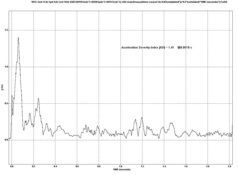
Figure 7-16. Test 671 Acceleration Severity Index Vs Time
