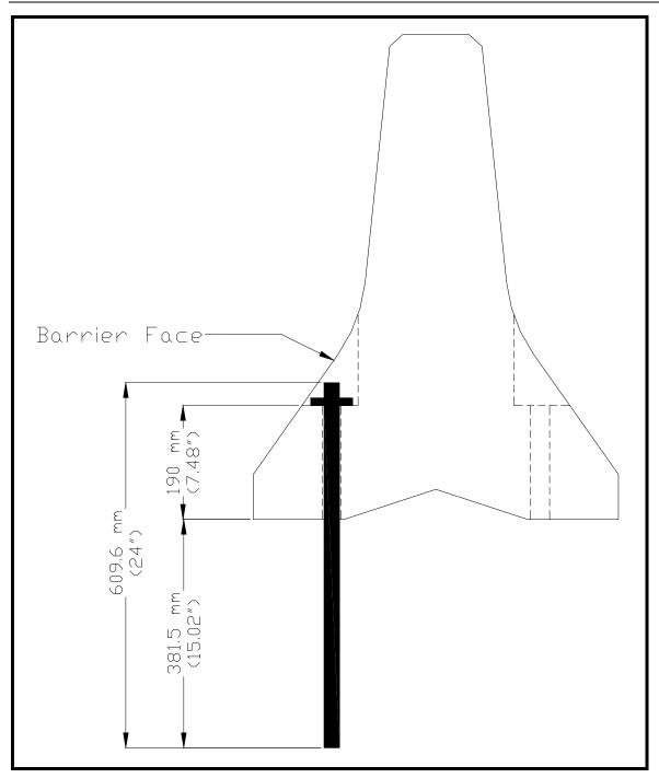
Figure 7-5. Typical Capped Stake Installation Layout
