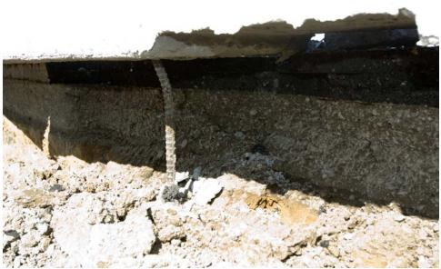
Figure 2-54. Test 674 - Damaged Pavement from Rear Stake
