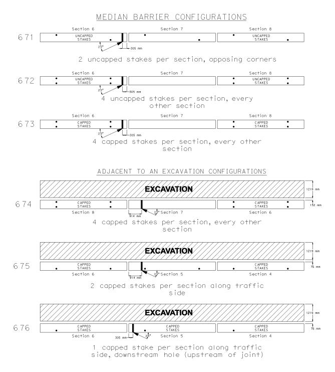
Figure 2-5. Staking Configurations Layout
