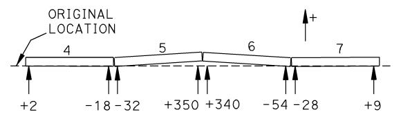
Figure 2-63. Test 675 - Barrier Static Displacements [mm]
