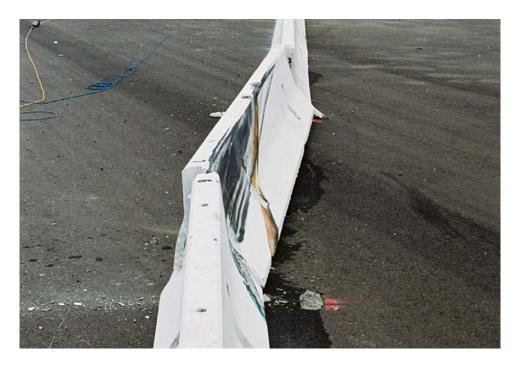
Figure 2-11. Test 671 - Downstream View of Barrier Post-Impact
