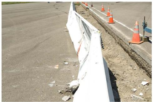
Figure 2-77. Test 676 - Downstream View of Barrier Post-Impact
