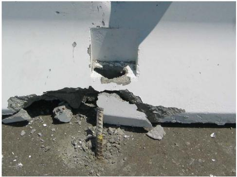
Figure 2-13. Test 671 - Section 6 Upstream Stake Post-Impact
