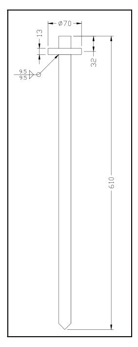
Figure 7-6. Capped Stake Dimensions [mm]
