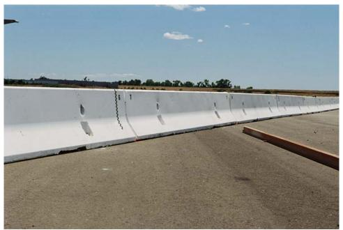
Figure 2-9. Test 671 - Barrier Pre-Impact
