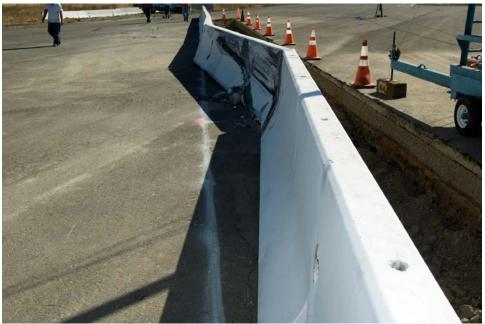
Figure 2-50. Test 674 - Downstream View of Barrier Post-Impact
