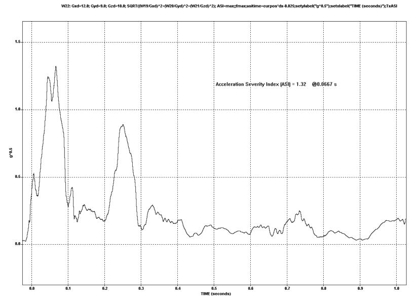
Figure 7-33. Test 675 Acceleration Severity Index Vs Time
