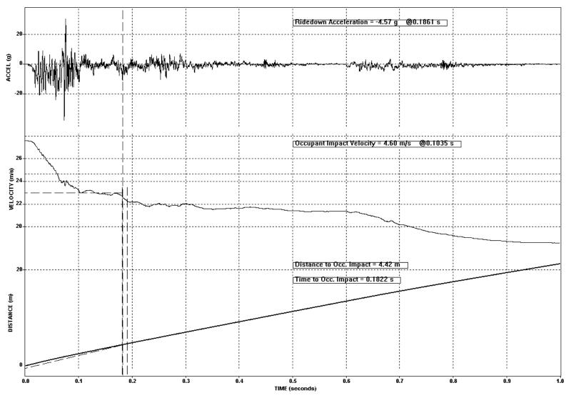
Figure 7-19. Test 672 Vehicle Longitudinal Acceleration, Velocity, and Distance Vs Time
