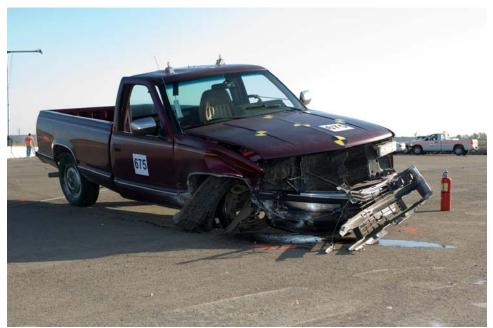
Figure 2-70. Test 675 - Front-right View of Vehicle Post-Impact
