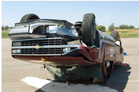
Figure 2-80. Test 676 - Vehicle Post-Impact Front View
