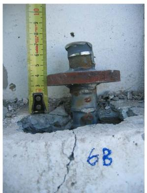
Figure 2-39. Test 673 - Stake #6B Post-Impact
