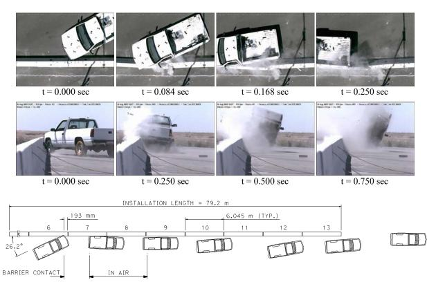
Figure 2-43. Test 673 - Impact sequence and diagram
