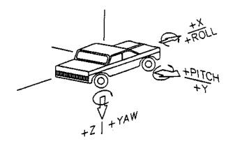
Figure 7-12. Vehicle Accelerometer and Gyro Sign Convention
