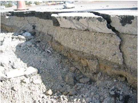
Figure 2-55. Test 674 - Pavement Damage after Barrier Removal
