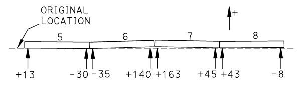
Figure 2-36. Test 673 - Barrier Static Displacements [mm]
