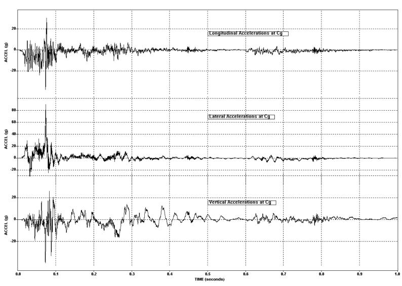
W11: Test 672 - k-rail staking Configuration 2, Longitudinal, Lateral and Vertical Accelerations
