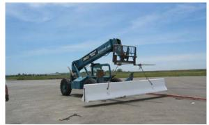
Figure 7-8. Forklift Carrying K-rail
