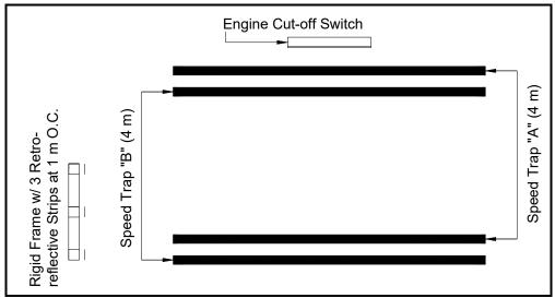
Figure 7-11. Instrumentation Layout
