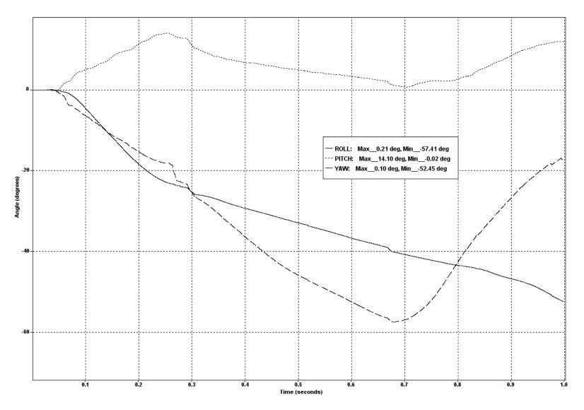
Figure 7-41. Test 676 Vehicle Roll, Pitch, and Yaw Vs Time
