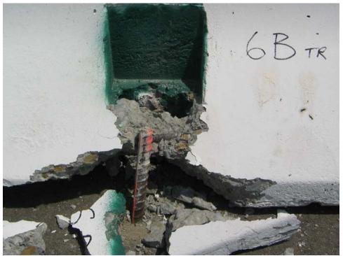
Figure 2-26. Test 672 - Stake #6B Post-Impact
