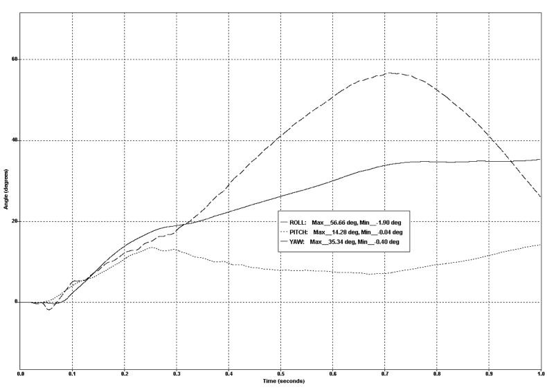
W15: Test 672 - k-rail staking Configuration 2, Roll Pitch and Yaw Angles
