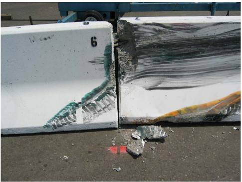
Figure 2-25. Test 672 - Impact Point Post-Impact
