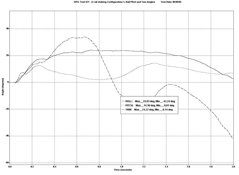
Figure 7-17. Test 671 Vehicle Roll, Pitch, and Yaw Vs Time
