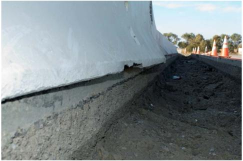
Figure 2-65. Test 675 - Barrier over Excavation
