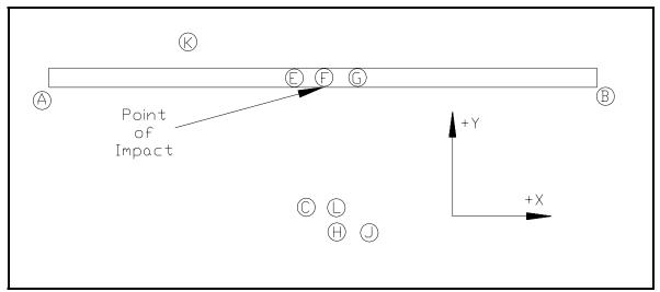
Figure 7-2. Typical Camera Locations and Labels
