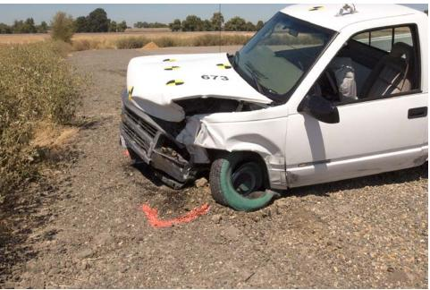
Figure 2-41. Test 673 - Front-left View of Vehicle Post-Impact
