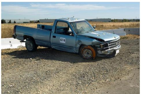
Figure 2-56. Test 674 - Side View of Vehicle Post-Impact
