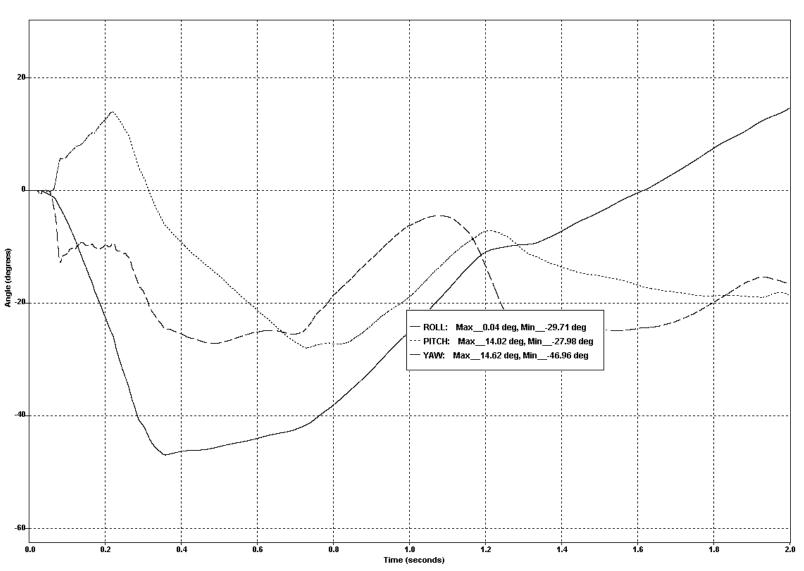
W15: Test 674 - k-rail staking Configuration 4, Roll Pitch and Yaw Angles
