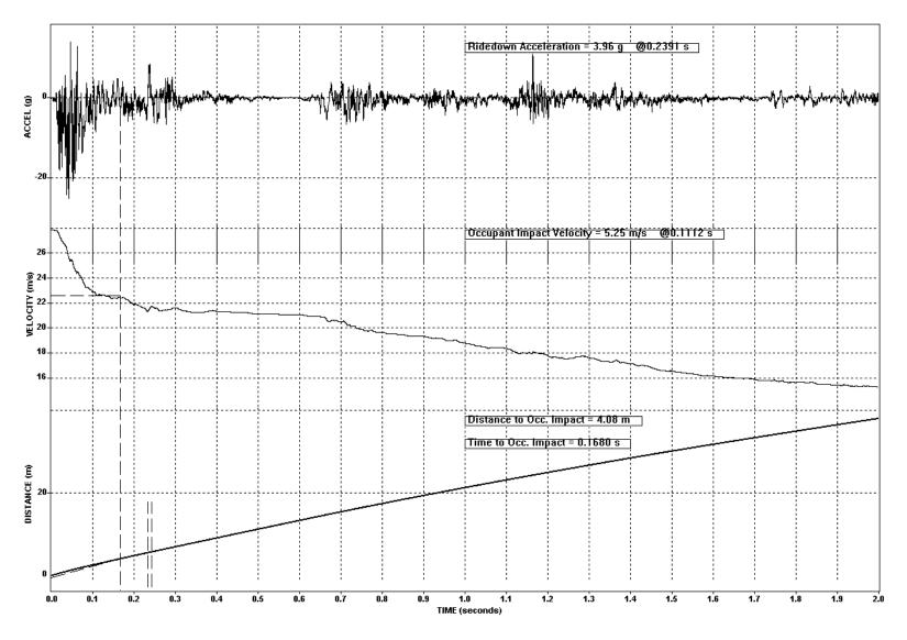
Figure 7-14. Test 671 Vehicle Longitudinal Acceleration, Velocity, and Distance Vs Time
