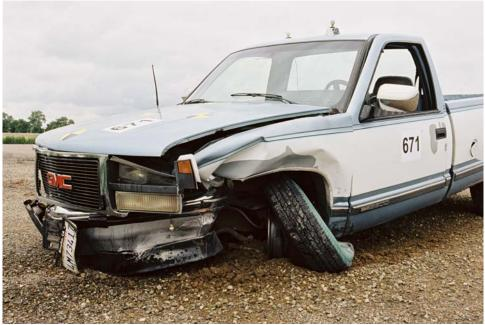
Figure 2-15. Test 671 – Front-left View of Vehicle Post-Impact
