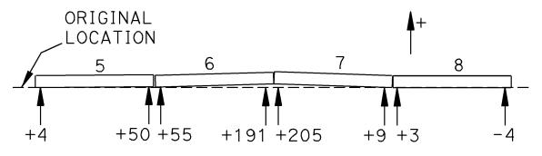
Figure 2-23. Test 672 - Barrier Static Displacements [mm]
