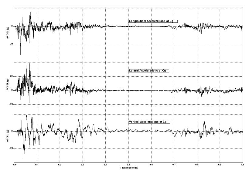
W11: Test 676 - k-rail staking Configuration 6, Longitudinal, Lateral and Vertical Accelerations
