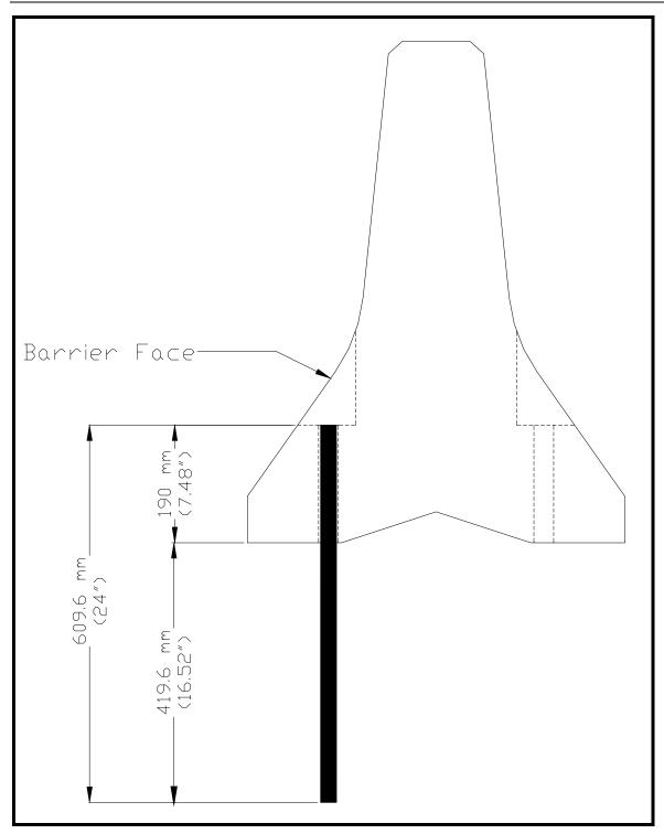
Figure 7-4. Typical Uncapped Stake Installation Layout
