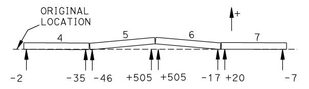
Figure 2-76. Test 676 - Barrier Static Displacements [mm]
