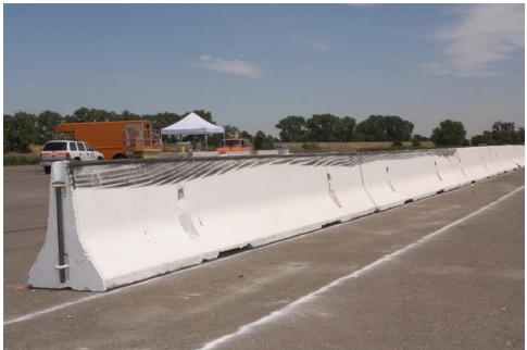
Figure 2-27. Test 672 - Scuffing on the Backside of the Barrier
