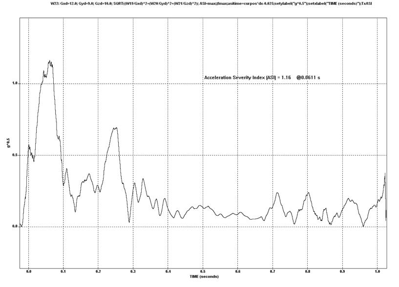
Figure 7-42. Test 676 Acceleration Severity Index Vs Time
