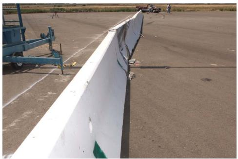
Figure 2-24. Test 672 - Downstream View of Barrier Post-Impact
