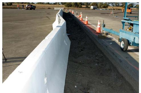
Figure 2-64. Test 675 - Downstream View of Barrier Post-Impact
