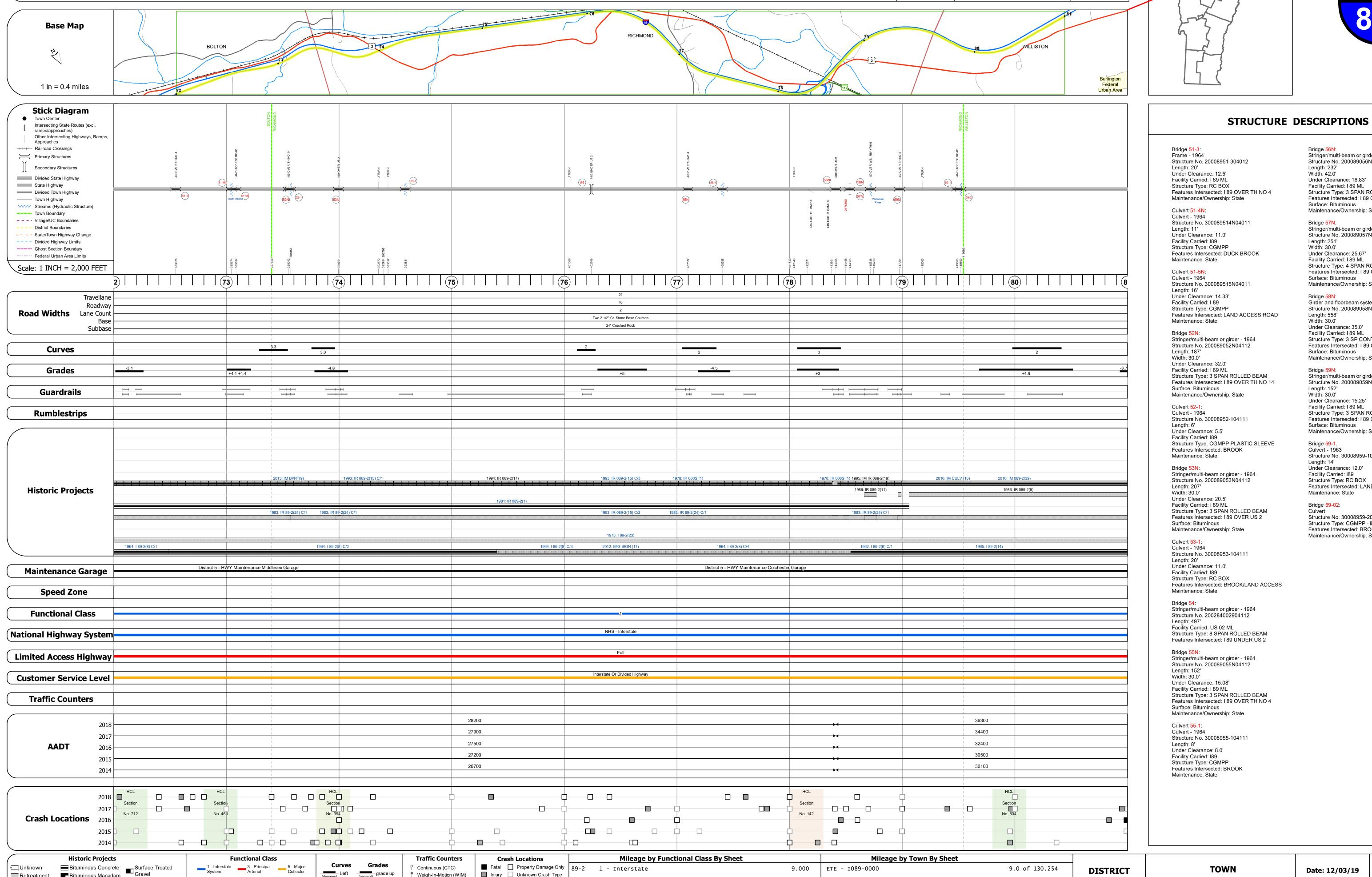
Stringer/multi-beam or girder - 1964 Structure No. 200089056N04112 Length: 232' Width: 42.0' Under Clearance: 16.83' Facility Carried: I 89 ML Structure Type: 3 SPAN ROLLED BEAM Features Intersected: I 89 OVER US 2 Surface: Bituminous Maintenance/Ownership: State Bridge 57N: Stringer/multi-beam or girder - 1964 Structure No. 200089057N04112
