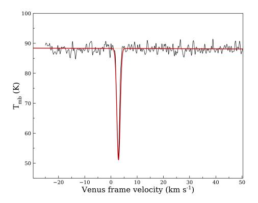
Figure 3: Absorption spectram of CH<sub>3</sub>CH<sub>2</sub>CN (J=29(12,17)–28(12,16)) at  $\nu$ =259.869 GHz with single gaussian fitting (FWHM=0.73±0.02 km s<sup>-1</sup>). The spectrum was made by integrating the reduced ALMA data cubes from the centre of Venus (12579.1 km at Venus' distance) within a circular region of 25.2" diameter. The continuum emission of Venus is subtracted from the spectrum.
