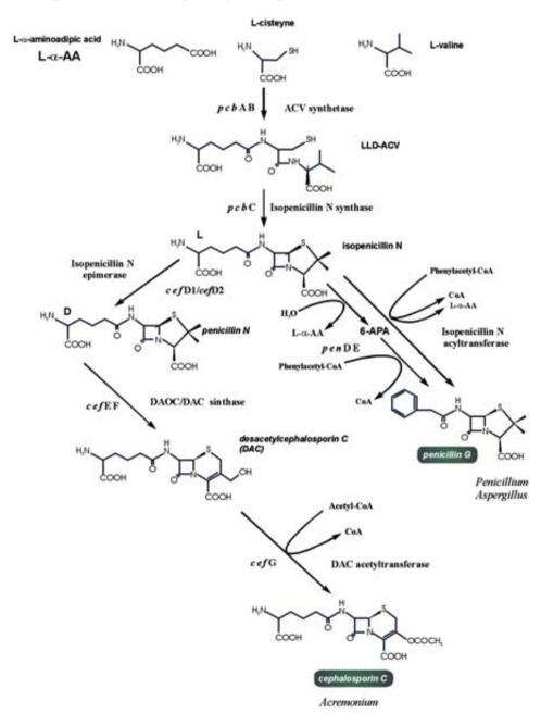
Figure 2. Biosynthetic pathways for penicillin and cephalosporin.
