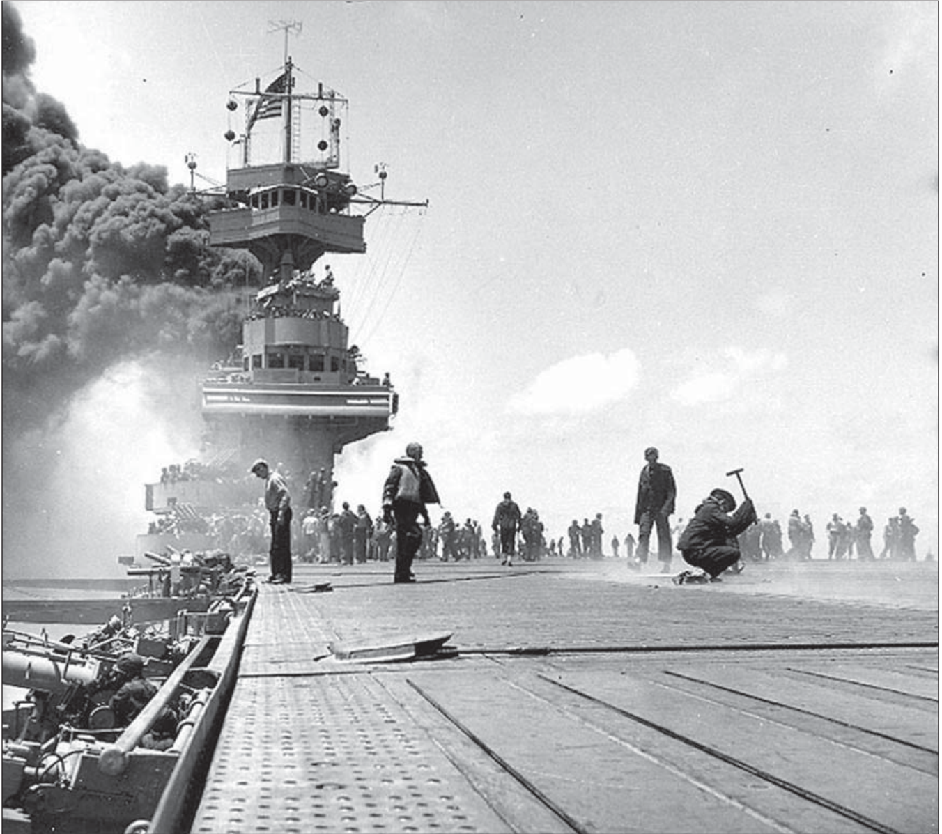
The USS Yorktown during the Battle of Midway, June 1942, shortly after being hit by three Japanese bombs. Man with hammer at right is probably covering a bomb entry hole in the forward elevator. U.S. Navy photograph at U.S. National Archives
