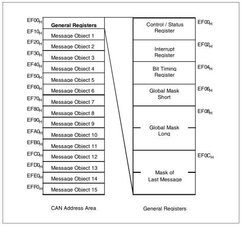
Figure 9 CAN addressing area on the C167CR
