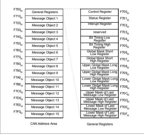
Figure 8 CAN addressing area on the C515C
