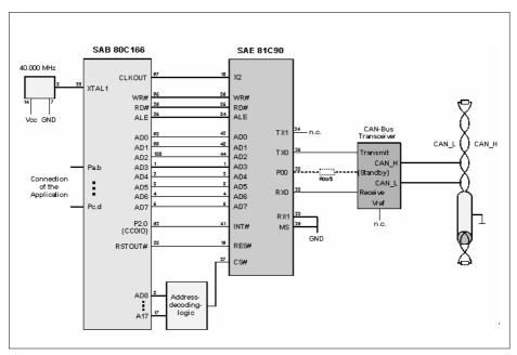
Figure 15 Connection of a SAB 80C166 to CAN via the SAE 81C90 (parallel)
