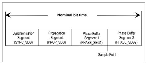
Figure 5 Partition of bit time
