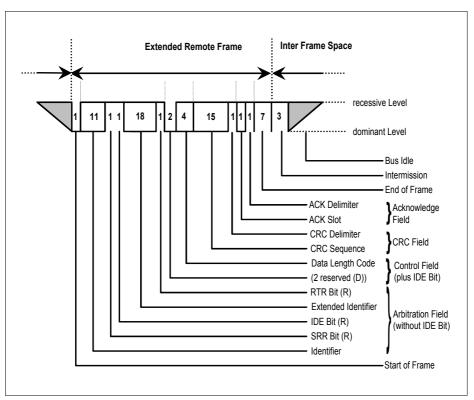
Figure 4 Extended CAN Remote Frame
