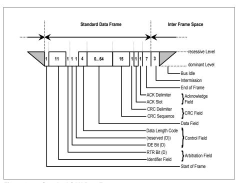
Figure 1 Standard CAN Data Frame
