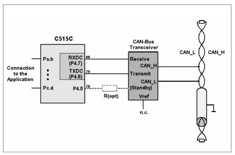
Figure 14 Connection of a C515C to CAN
