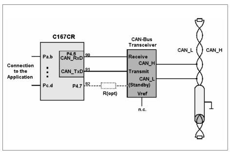
Figure 13 Connection of the C167CR to CAN
