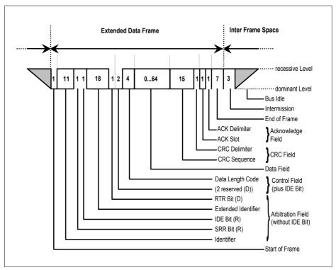
Figure 2 Extended CAN Data Frame
