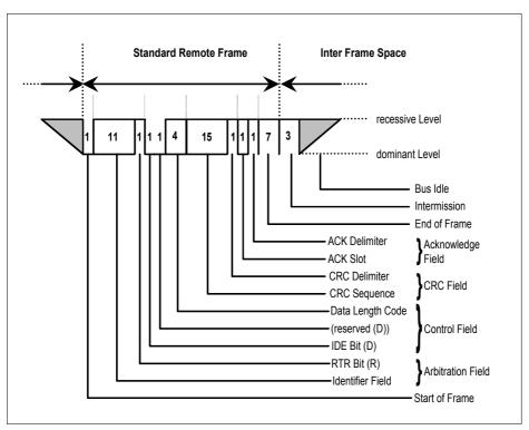
Figure 3 Standard CAN Remote Frame
