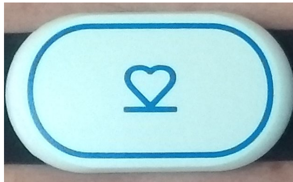
Figure 28: The heart symbol indicating the correct orientation of the sensor.
