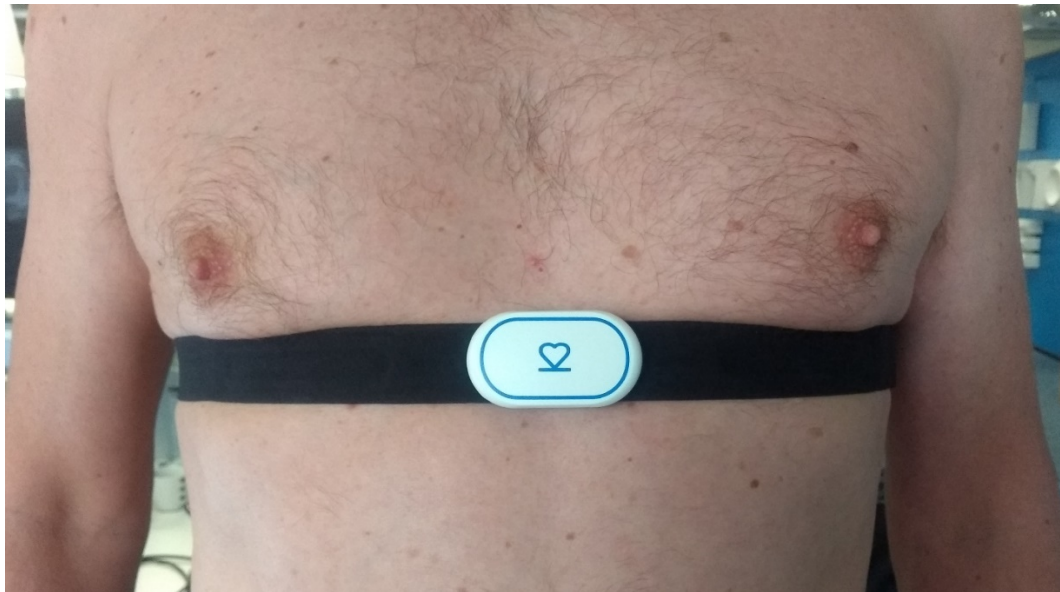
Figure 1: The Beat2Phone sensor properly attached to chest with the electrode strap.
