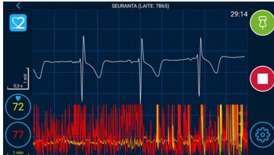
Figure 25: The sensor is upside down in the electrode strap.
