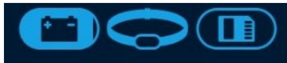
Figure 11 From left to right: sensor battery status, leads on/off, sensor memory status
