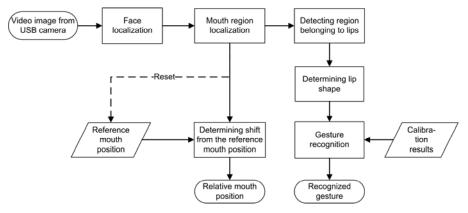
Fig. 2. Scheme of the LipMouse human-computer interface algorithm
