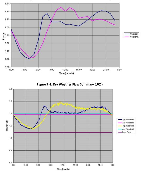
Figure 7.3: Dry Weather Flow Diurnal Peak Factors (UC1)
