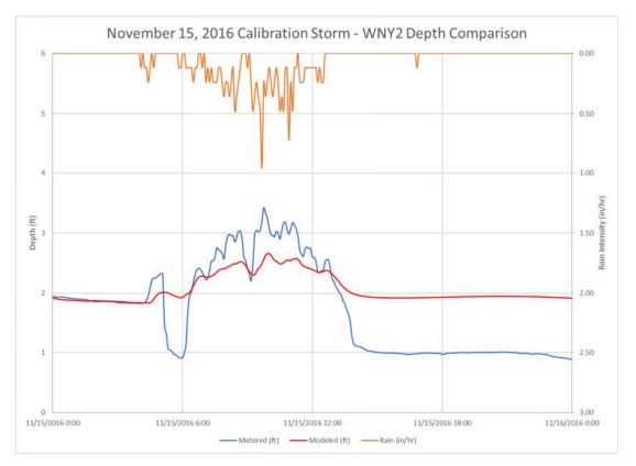
Figure 8.17 November 15, 2016 Calibration Storm Flow Depths (WNY2)
