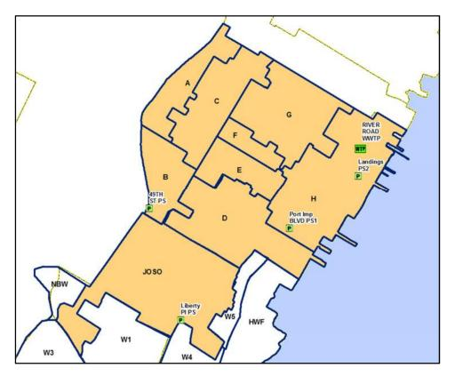
Figure 6.1: Basins within the River Road WWTP Service Area
