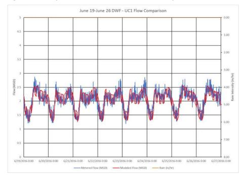
Figure 8.7: Comparison of Measured vs. Simulated Dry Weather Flows (UC1)
