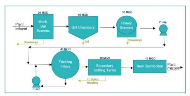
Figure 5.1: River Road WWTP Process Flow Diagram
