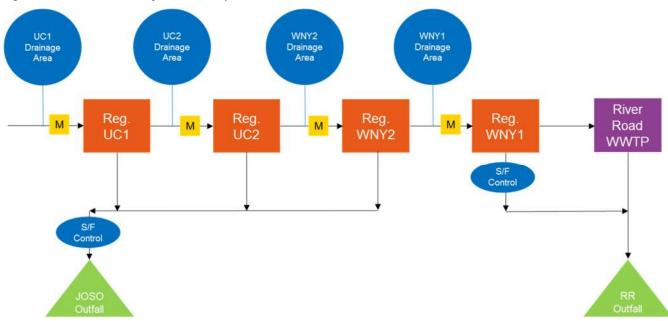
Figure 2.3: Flow Schematic of River Road System
