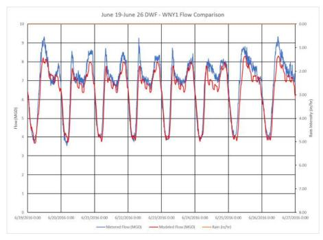
Figure 8.9 Comparison of Measured vs. Simulated Dry Weather Flows (WNY1)
