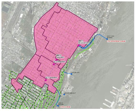
As can be seen in the schematic above, the regulators are located in series along the main WNY interceptor sewer, and one meter was located upstream of each regulator prior to the flow split. As such, the meter upstream of the UC1 regulator is the only meter not impacted during wet weather by the hydraulic performance of the other regulators.
