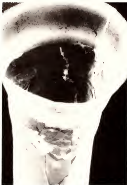
Fig. 2. Radiograph of the added rim section showing seams and differences in density between the horn and rim.
