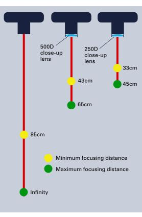
Close-up lenses work by decreasing the minimum focus of your lens. With a close-up lens fitted you can move the camera lens closer to your subject and gain a higher level of magnification.
