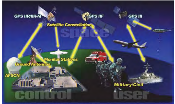
AFSCN – Air Force Satellite Control Network GPS IIR – Global Positioning System (GPS) Block II “Replenishment” Satellites GPS IIR-M – GPS Block II “Replenishment – Modernized” Satellites GPS IIF – GPS Block II “Follow-On” Satellites GPS III – GPS Block III Satellites
