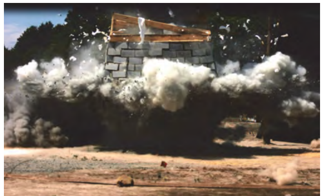
Figure 3. Concrete masonry unit for characterizing building debris
