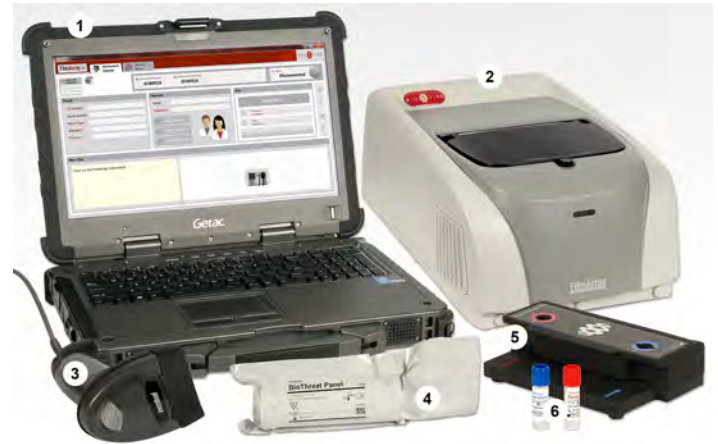
1 - Laptop running NGDS software 2 - NGDS PCR (Polymerase Chain Reaction) instrument 3 - Barcode reader 4 - Assay Panel (in bag) 5 - Assay Panel Docking Station 6 - Hydrating Solutions
