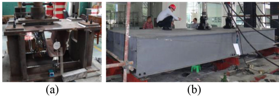
Fig. 14 Full-scale test of OSDs with TEUs: a Rib-to-deck specimen; b Segment specimen
