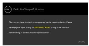
This means that the monitor cannot synchronize with the signal that it is receiving from the computer. See Monitor Specifications for the Horizontal and Vertical frequency ranges addressable by this monitor. Recommended mode is 3840 x 2160.
