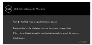
If either HDMI,DP, USB Type-C input is selected and the corresponding cable is not connected, a floating dialog box as shown below appears.
