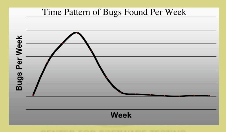
This curve is used to predict ship dates and to signal when a milestone has or has not been met. The predictions are based on fitting bug counts to a Weibull curve. What's the rationale?
