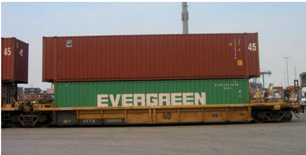
Figure 27. Double-stack container traffic: 45' container stacked atop a 40' container on 40' articulated well wagon
