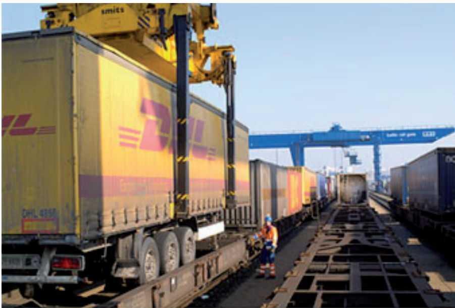
Figure 41. 45' piggyback trailer in Europe
