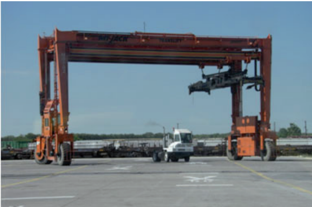
Figure 48. Rubber-tyred Gantry Crane and terminal tractor (tugmaster)
