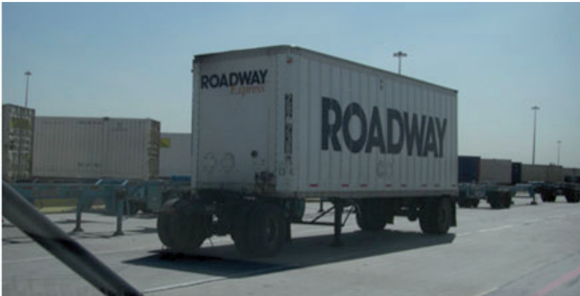
Figure 43. 28' piggyback trailer in North America
