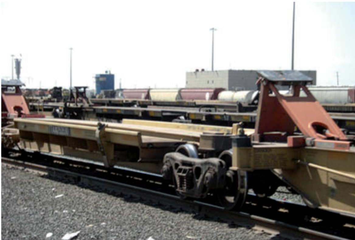
Figure 36. TTX spine wagon for carrying trailers
