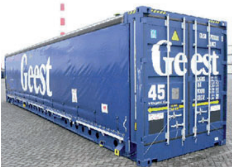
Figure 39. 45’ curtainsider domestic container in Europe
