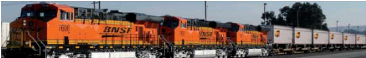
Figure 10. U.S. intermodal technology: trailer on flatcar
