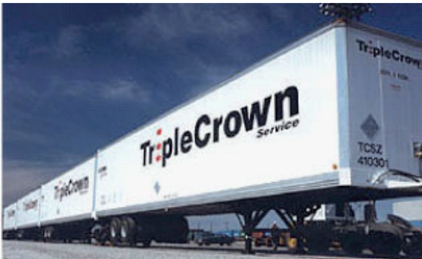
Figure 11. U.S. intermodal technology: RoadRailer
