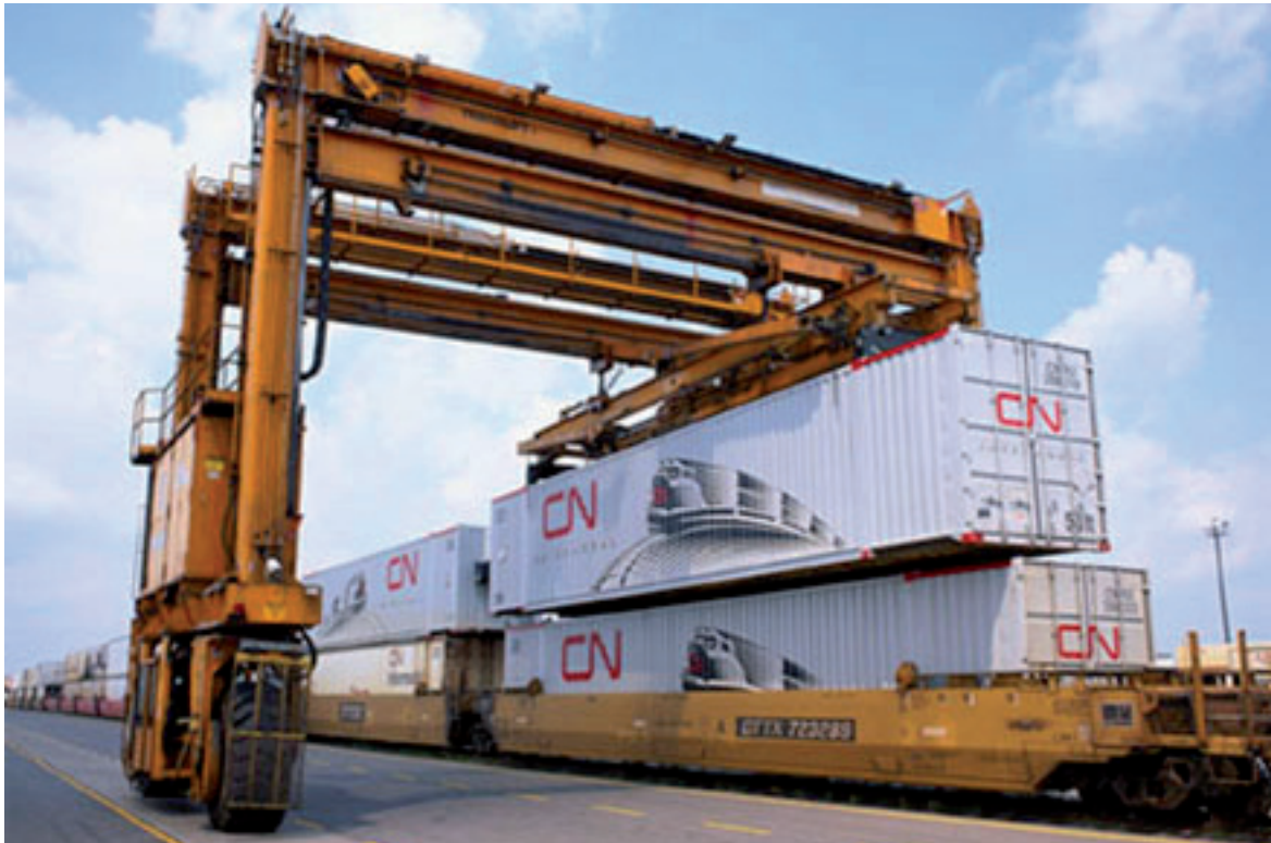
Figure 37. 53' domestic container in North America
