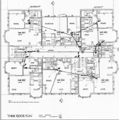
Fig. 87 – Plans from 1988 permit drawings, showing revised unit interior configurations constructed that year. Dark overlay lines represent the proposed electrical design. North is oriented down. (SDCI)
