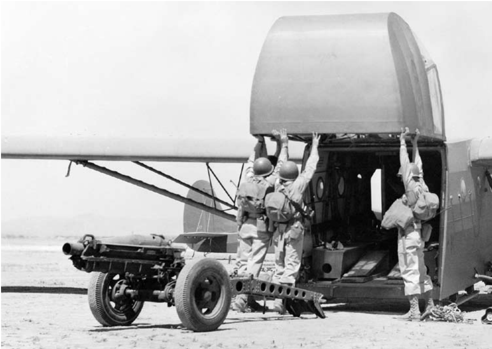
Airborne troops loading a 75-mm. pack howitzer into a cargo glider during training
