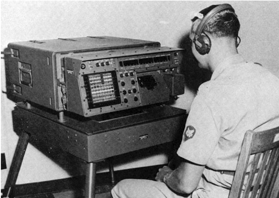
M18 field artillery digital automatic computer, commonly known as FADAC
