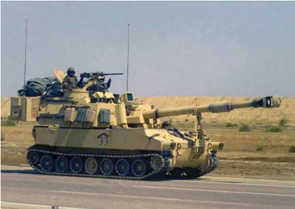
M109A6 self-propelled 155-mm. howitzer (Paladin) moving toward the Euphrates River during Operation IRAQI FREEDOM
