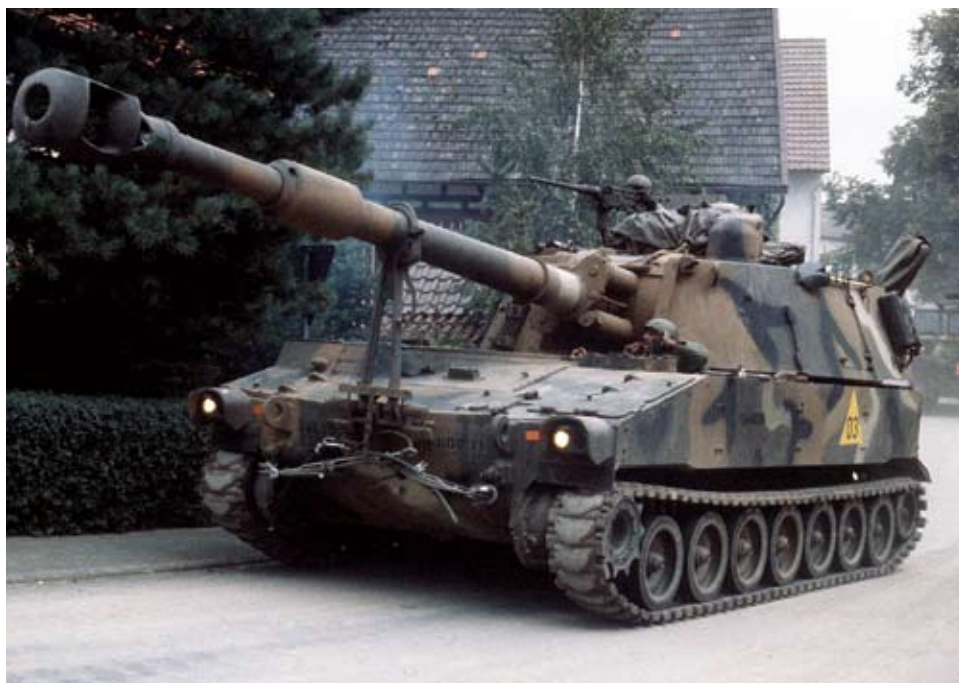
M109 self-propelled 155-mm. howitzer passing through a German town during a 1983 exercise
