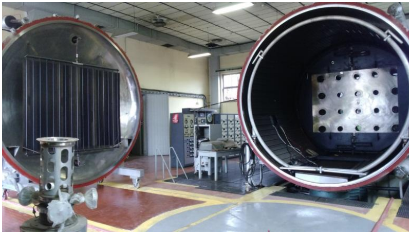
Figure 23 –Reverberation chamber; aperture diameter 3.5 m
