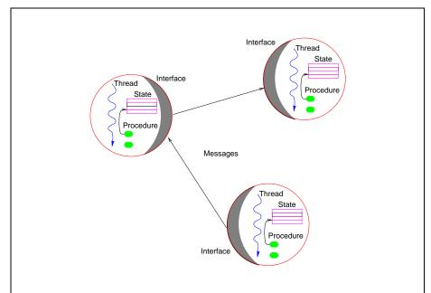
Figure 1: Actors encapsulate a thread and state. The interface is comprised of public methods which operate on the state.
