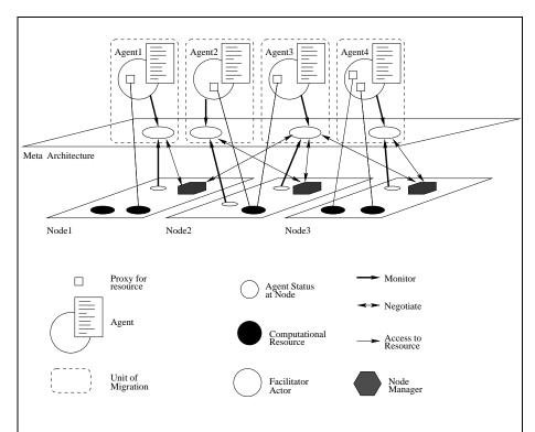
Figure 4: Agent System Architecture: Agent carries dynamic specification of its requirements from the computational environment
