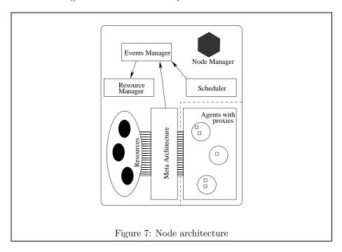
Every node has a node manager that serves as the contact agent for negotiating terms under which an agent may arrive and compute at the node. A contract determines the rate at which an agent would be charged for various resources, possibly depending on the state of the node, and is represented by a list of such functions. Note that there will be separate functions for time/space of usage of a resource, and for the guaranteed needed for the degree of access to the resource.
