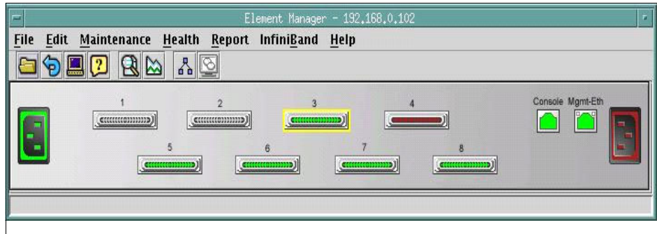
Figure 6-1 How check port states in Cisco Element Manager
