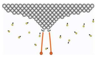
Fig. 4. Spherical tip after the atoms have been rearranged to form a three-sided pyramid. Now the ionization disks exist only over the topmost three atoms. Reprinted with permission from Ward B.W., Notte J.A. & Economou N.P., 2006. Helium ion microscope: A new tool for nanoscale microscopy and metrology. JVST B 24(6), 2871. Copyright 2006, American Vacuum Society.
