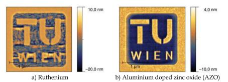
Fig. 15. AFM images of two hard materials after pattern definition. The patterning process was identical; however, the resulting pattern quality differs significantly. The nominal hard mask thickness before patterning was 10 nm in both cases.
