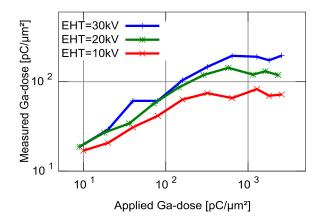
Fig. 10. Impact of the applied Ga dose on the effectively implanted ion dose. The indicated measured ion dose shown was calculated from the measured relative ion dose as described in the text.
