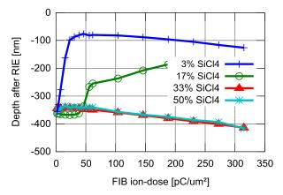
Fig. 17. Impact of the addition of SiCl<sub>4</sub> to the masking capability of Ga implanted by FIB into Si in a SF<sub>6</sub>-based RIE process
