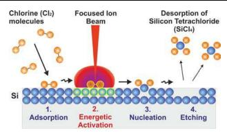
Fig. 7. Schematic illustration of the FIB-induced etching process
