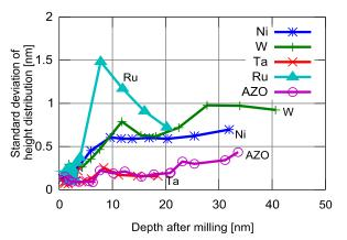
Fig. 16. Impact of ion milling on the roughness of hard mask materials. The hard mask thickness before milling was 10±2 nm in all cases.
