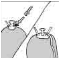
Fig 1 Remove plastic nut and nozzle (may require wrench or pliers). Attach tubing to nipple on tank valve
