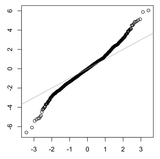
In contrast to Figure 2-11, the points are far below the line for low values and far above the line for high values. This means that we are much more likely to observe extreme values than would be expected if the data had a normal distribution. Figure 2-12 shows another common phenomena: the points are close to the line for the data within one standard deviation of the mean. Tukey refers to this phenomenon as data being "normal in the middle," but having much longer tails (see [Tukey-1987]).
