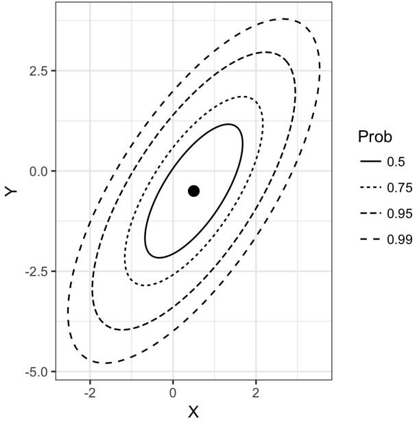
Figure 7-9. Probability contours for a two-dimensional normal distribution
