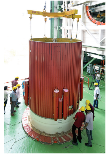
Placement of interstage over PSLV-C46 first stage during vehicle integration
