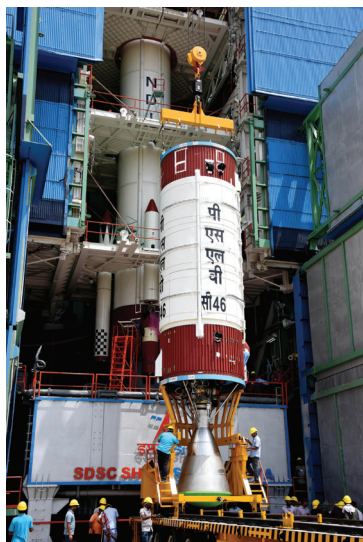
Hoisting of PSLV-C46 Liquid second stage
