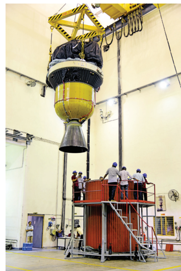
PSLV-C46 Third and Fourth stages at Stage preparation Facility
