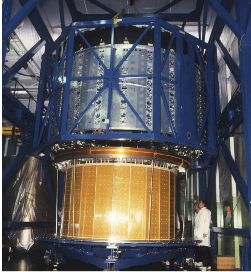
Fig. 20: DELPHI RICH detector being inserted into the mirror's barrel.
