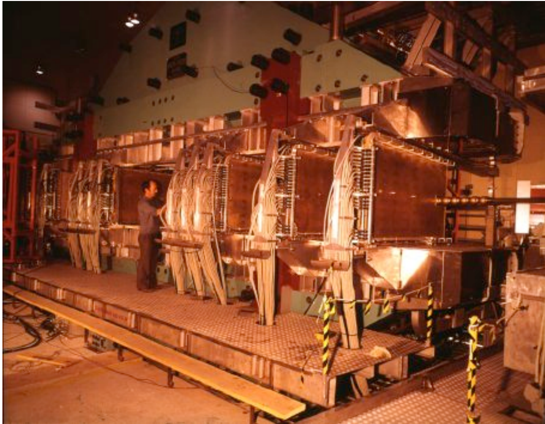
Fig. 5: The Split Field Magnet detector, mounting a set of large MWPCs.
