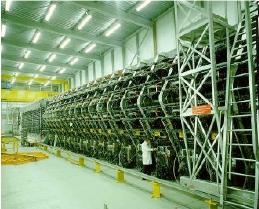
Fig. 6: The WA1 neutrino experiment, using large area wire drift chambers.
