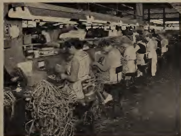
Shown above is one of the numerous Bally cable soldering lines at which the cables are secured to the connectors . . . "serpentine highways of wire for the tireless messengers of electric impulses."
