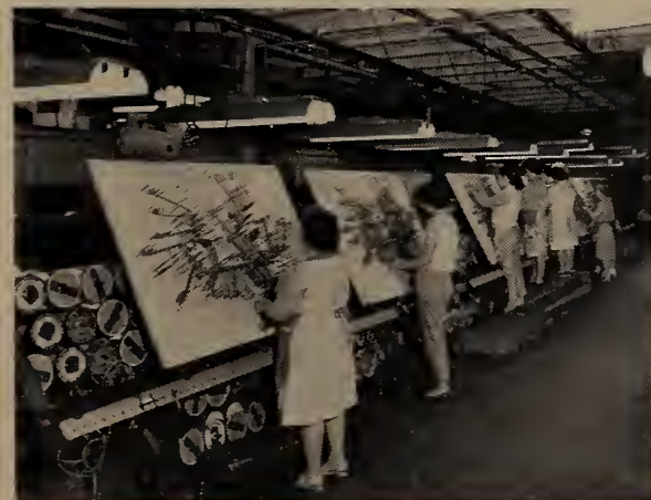
Photograph shows one of a dozen Bally cable forming lines where cables often containing 1,700 feet of wire in 45 different code colors are assembled by skilled women.
