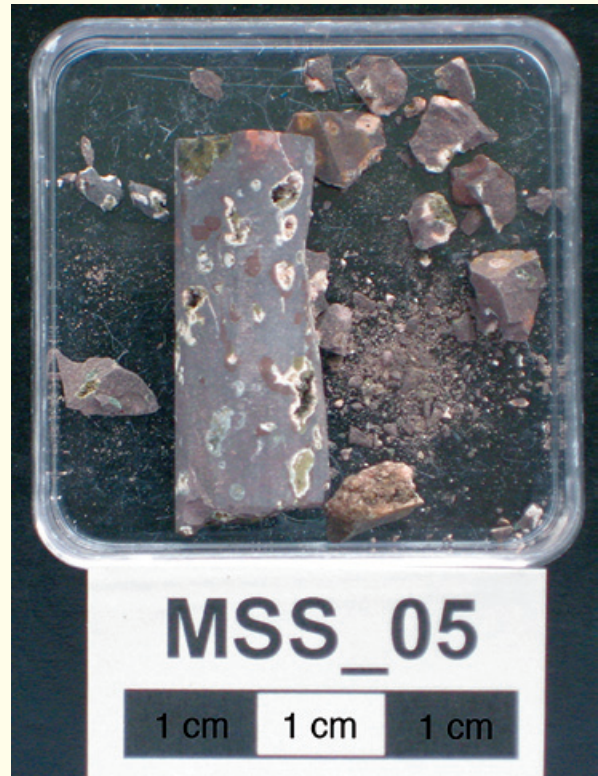
Figure 11. A Mars sample simulant (MSS) is a 10 g sample, intended to simulate the variety of material that could be returned from Mars in terms of shape, hardness and other properties affecting the handling of a sample. Credit: Dr. B. Hofmann, University of Berne
