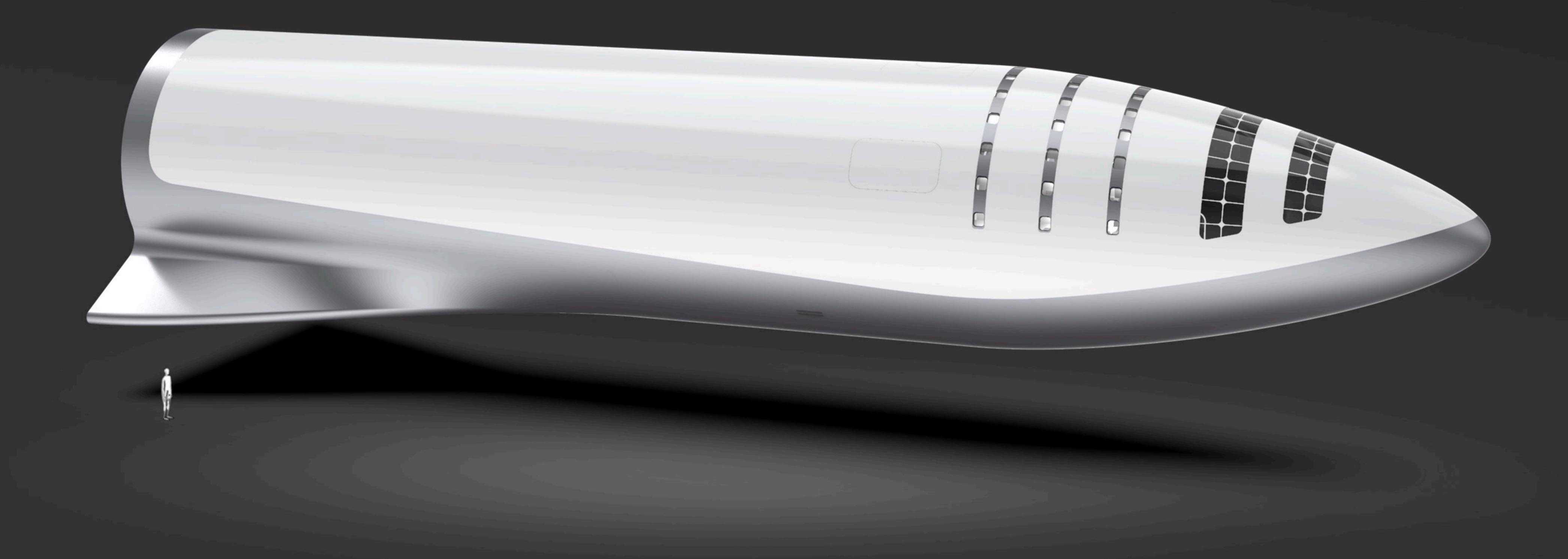
Ship Length 48 m Body Diameter 9 m Ship Dry Mass 85 t Propellant Mass 1,100 t Max Ascent Payload 150t Typical Return Payload 50 t
