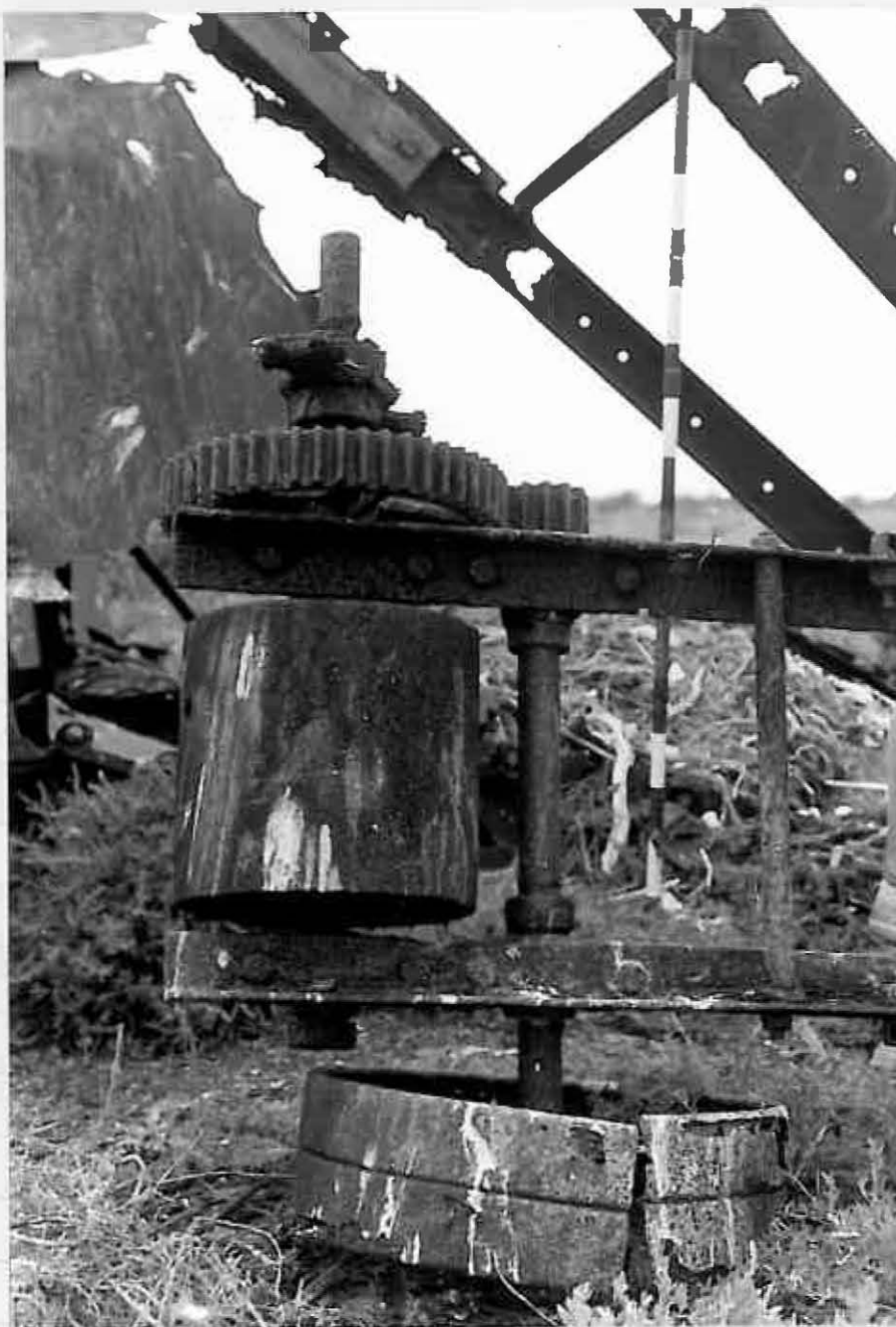
Remains of reduction gear of bucket elevator from steel guano bin, Pelsaert Island, October 1979
