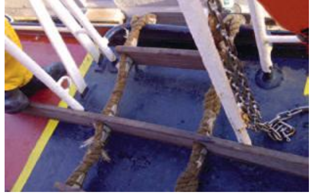
Poor and incorrect securing method
