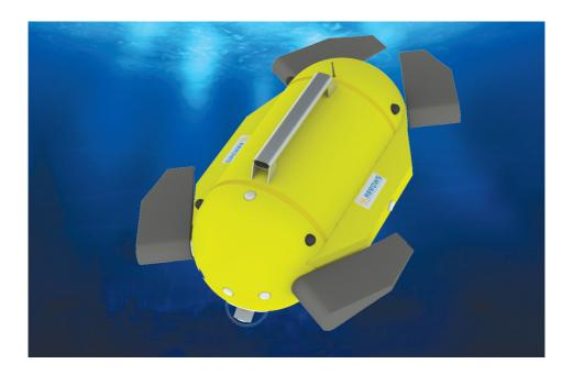
«Fin propulsors of U-CAT can drive the robot in all directions without disturbing water and beating up silt from the bottom, which would decrease visibility inside the shipwreck», says researcher Taavi Salumäe, the designer of the U-CAT concept.
