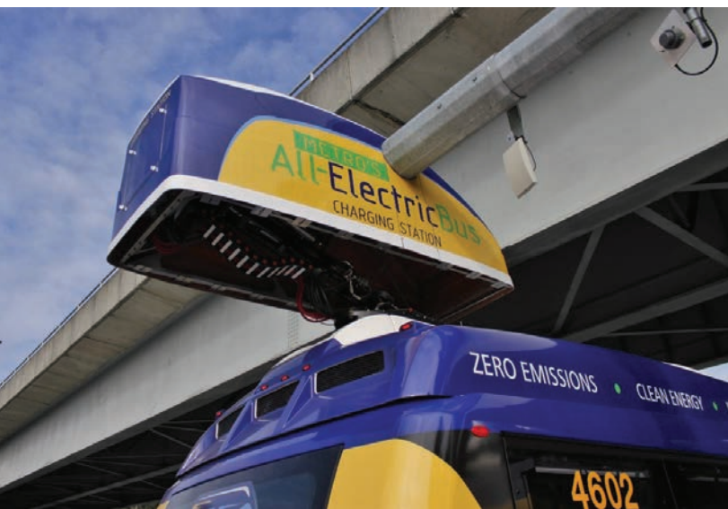
A King County Metro electric bus charging at Eastgate Park & Ride. Credit: SounderBruce via Flickr, CC BY-SA 2.0.
