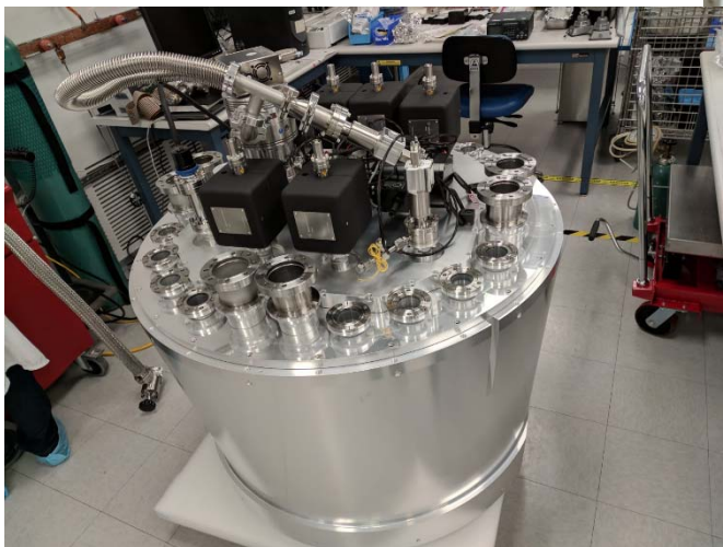
Cryostat During Leak Testing
