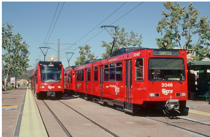
The Santee Town Center Green Line terminal in 2013, with a "long" 70-percent low-floor S70 to the left of a high-floor SD100.
