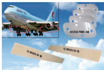
LE Splice and Access Panel
