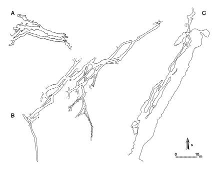
Fig. 7. Plans of typical horizontal caves in Turonian limestone in the Ayalon 1 region. Maze (network) pattern of conduits commonly develop along one or several bedding planes. Cave entrances are artificial. (A) 'Cave 4', coordinates 14349 14597; (B) Aneva Cave, 14347 14591, broken lines are elongated rifts at the bottom of passages (Fig. 9); (C) Zickron–Aneva Cave, 14310 14635.
