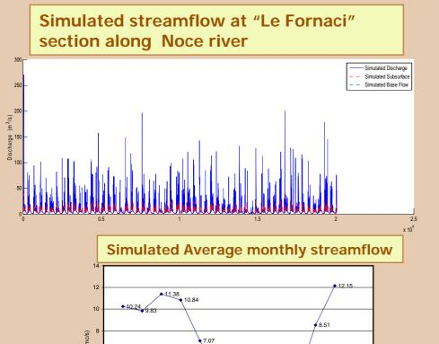
DREAM simulates the surface runoff, the subsurface runoff and the ground water contribution to streamflow
