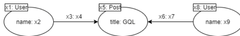
Figure 3.2: An example of a basic graph query searching for relationships between a specific post and users in a hypothetical graphical query language.
