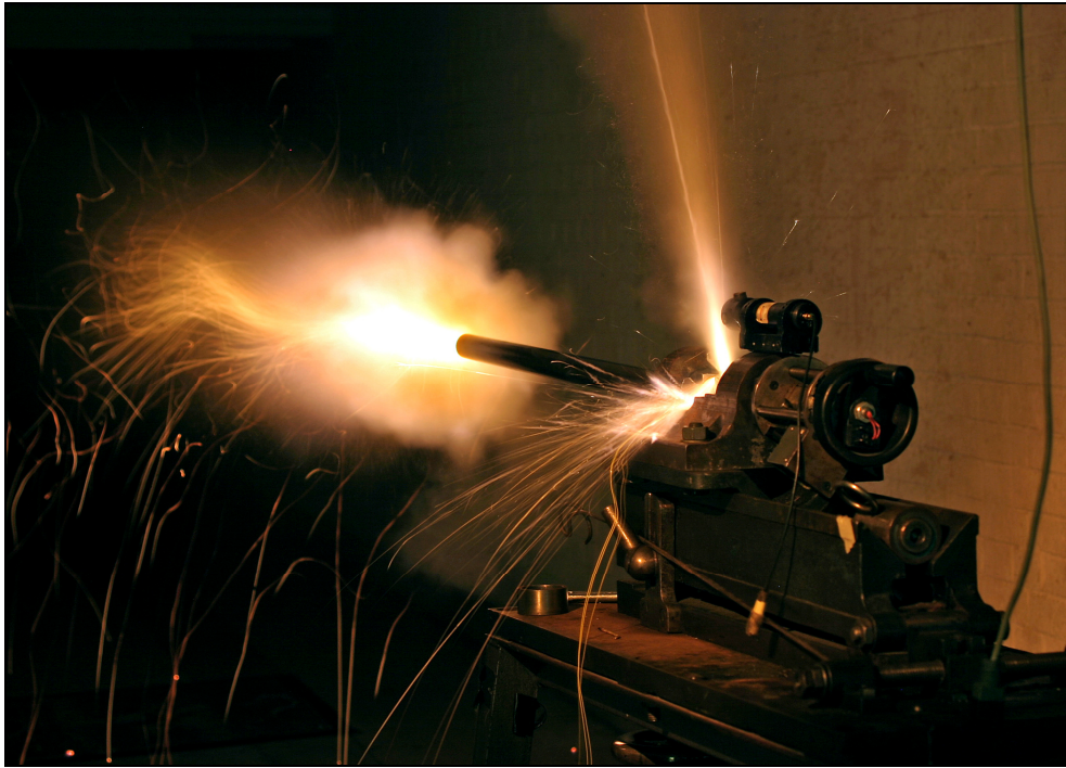
Figure 3.8: Firing experimental musket barrel
