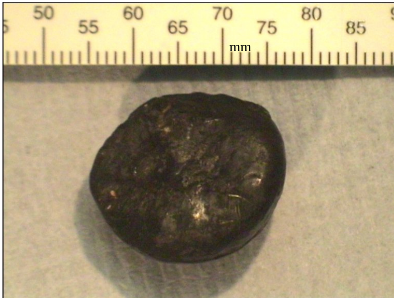
Figure 3.11: Damaged musket ball stopped in rubber shavings
