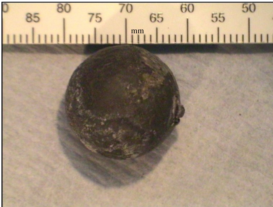
Figure 4.17: The recovered musket ball fired without a wad with a charge of 14 grams of G12 black powder
