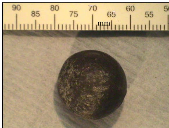
Figure 4.16: The recovered musket ball fired without a wad with 18 grams of G12 black powder from the 20.4 mm (large bore diameter) barrel
