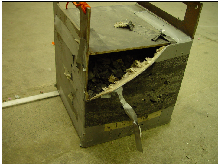
Figure 3.9: Steel box filled with shredded rubber. (Front cover partially removed to show shredded rubber)
