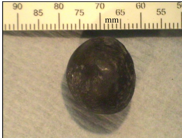
Figure 4.15: The recovered musket ball fired without a wad with 18 grams of G12 black powder from the 18.7 mm (small bore diameter) barrel
