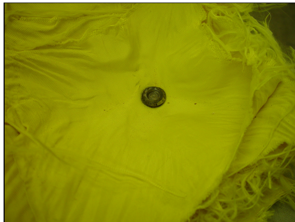
Figure 3.19: Captured solid slug in Kevlar
