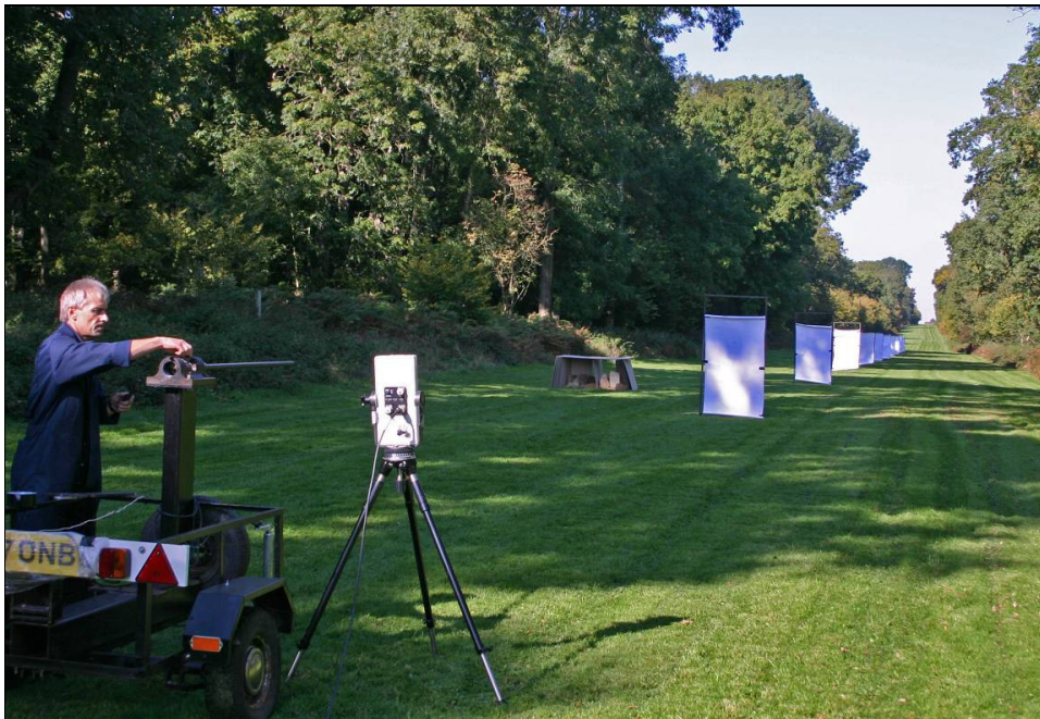
Figure 7.1: The view along Ashdown main ride showing the witness sheets at 20 m intervals to a distance of 200 m and with the number 3 housing and Doppler radar antenna for measuring projectile velocity
