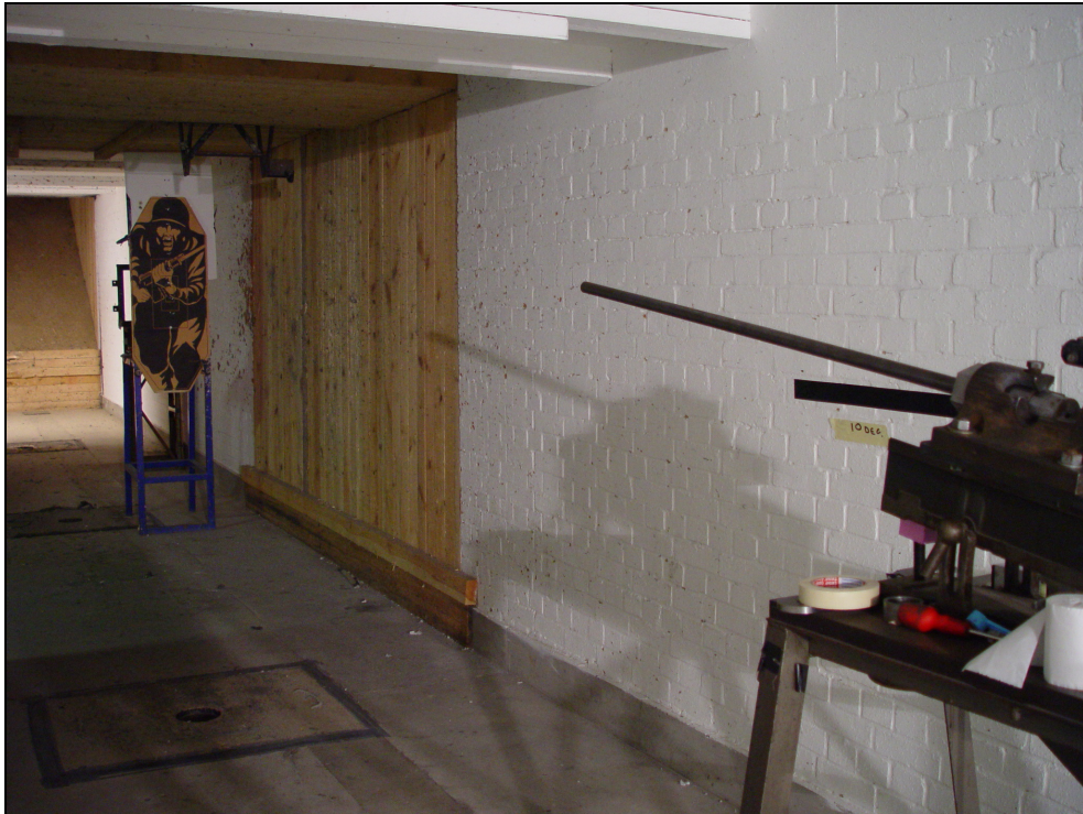
Figure 5.6: Proof mount with target showing elevation of the barrel
