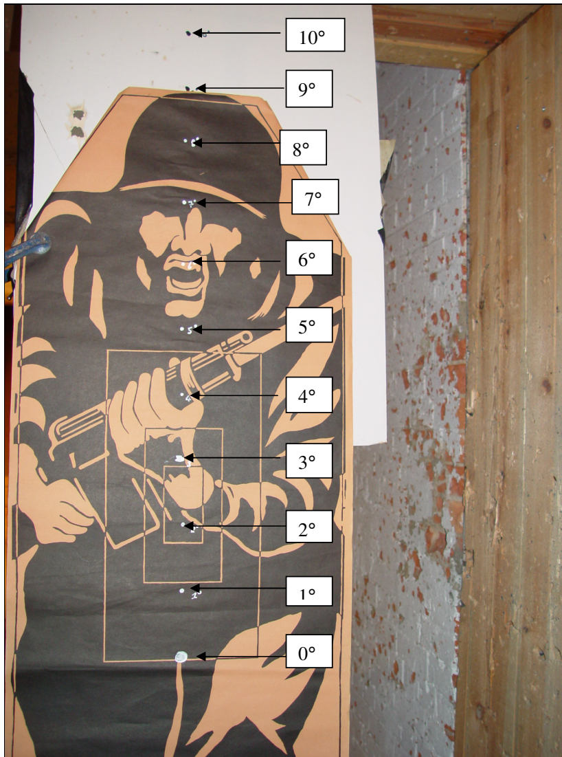
Figure 5.8: Impact positions from varying degrees of elevation upon a Figure 11 target placed five metres away from the muzzle
