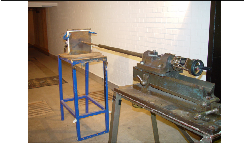
Figure 4.22: Arrangement used for investigating the effect of gas flow past the projectile by preventing movement of the musket ball by the use of a ram rod abutting against a fixed surface
