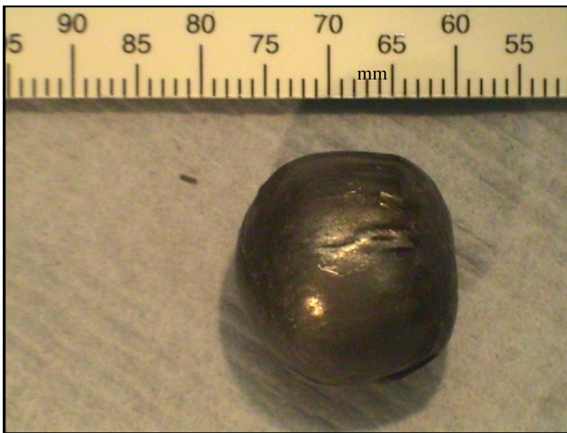
Figure 4.8: Retrieved Musket Ball from 12.5 grams of Swiss No.1 with wadding
