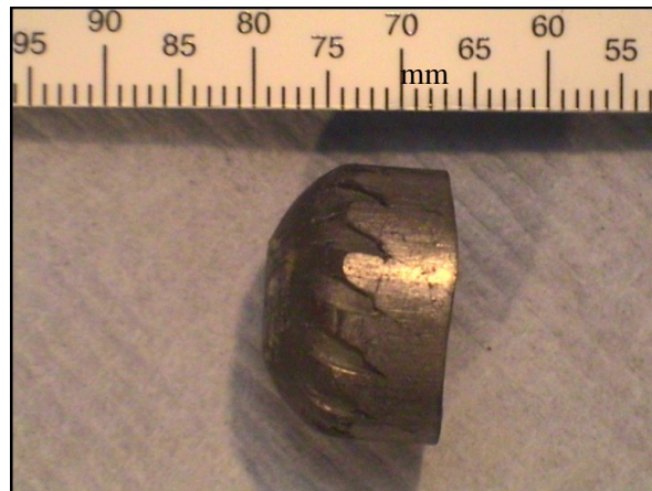
Figure 3.22: Solid slug retrieved from Plastozote and foam/Linotex
