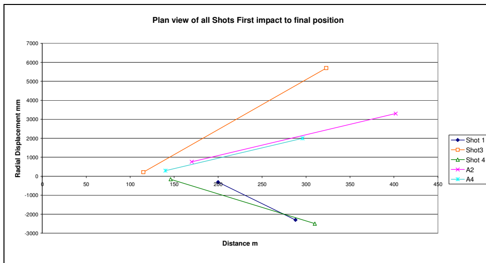
Figure 7.17: Final position of all recovered musket balls and their first impact point
