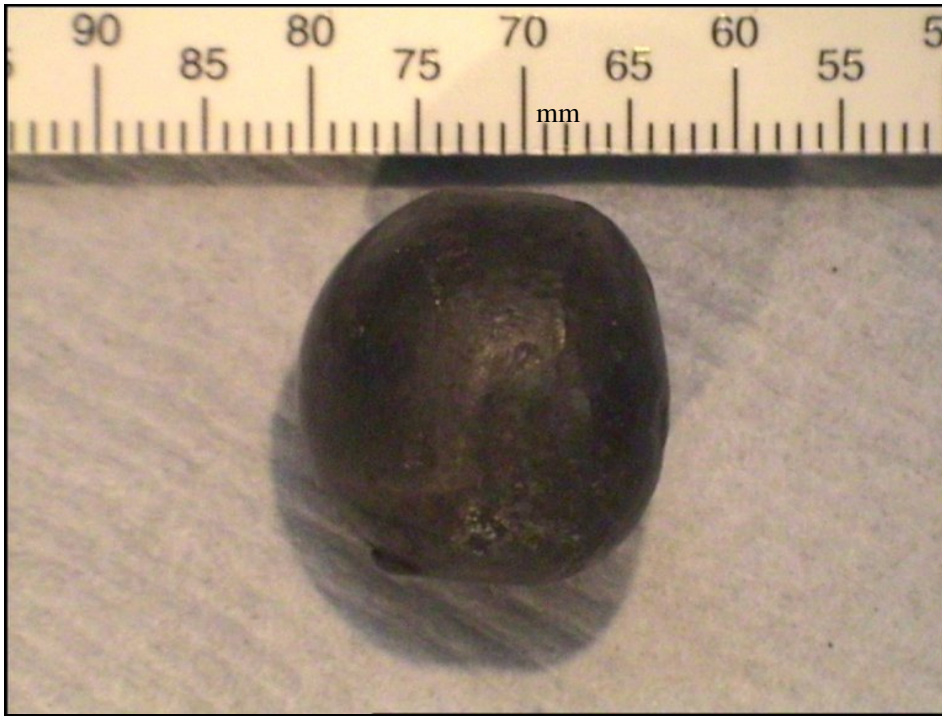
Figure 4.9: Retrieved Musket Ball from 12.5 grams G12 with wadding
