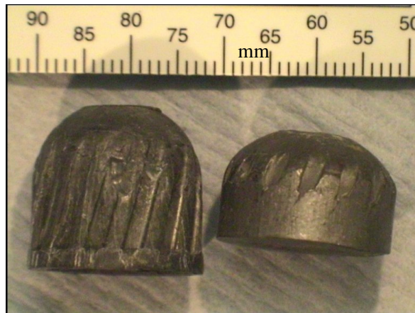
Figure 3.23 Solid slug before and after firing
