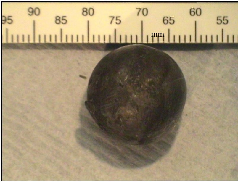
Figure 4.7: Retrieved Musket Ball from 12.5 grams of 3A with wadding
