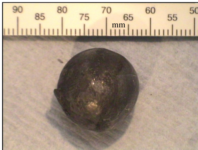
Figure 3.25: A typical retrieved musket ball that has successfully been captured by the soft capture system at 417 m/s using black powder
