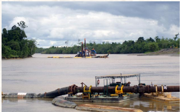
THE TAILINGS PROCESSING PLANT THAT IS PRODUCING A FINAL TAILING STREAM OF 1% SULPHUR AND SULPHIDE CONCENTRATE CONTAINING BETWEEN 42% AND 45% SULPHUR
