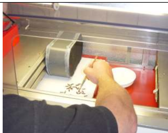
Fig. 15. Chiller, showing an emergence cage and adults immobilized by the cold.
