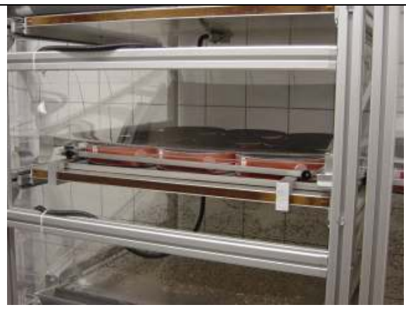
Fig. 12. TPU 3 feeding system with tray and heating plate, directly under cages. Two clips hold tray firmly onto the heating plate.
