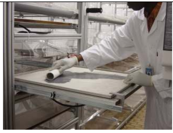
Fig. 10. Spreading blood with a paper roll, TPU 3 system.
