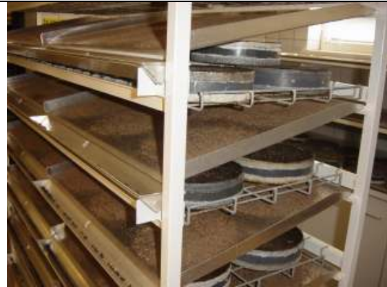
Fig. 2. Trolley showing sloped sheets and pupal-collecting trough.
