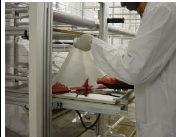
Fig. 9. Pouring blood onto a tray after lifting the membrane, TPU 3 system.
