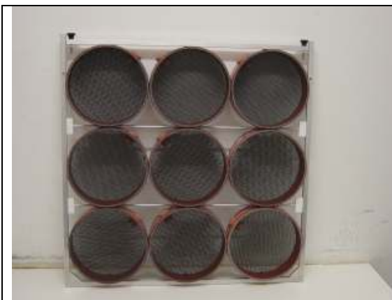
Fig. 5. TPU 3 cages (9) in a frame before being put into the TPU 3 system.
