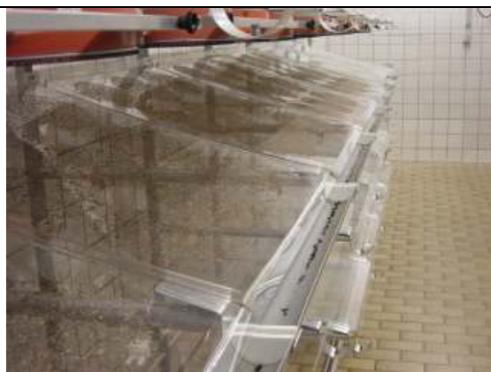
Fig. 6. TPU 3 sloped sheet below cages in frames, and pupal-collecting trough.
