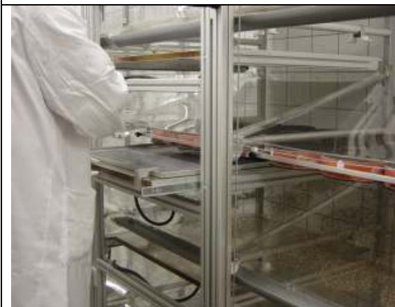
Fig. 11. Pushing tray with membrane and blood under a frame of cages, TPU 3 system.
