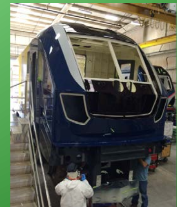
Carshell Final Paint
