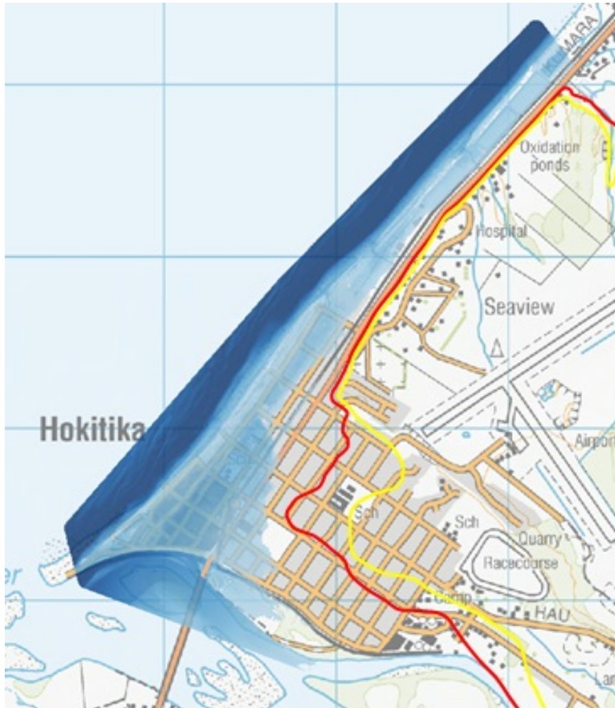
Figure 3.3: Hokitika - Estimated Inundation Area for 1:500 Tsunami Event
