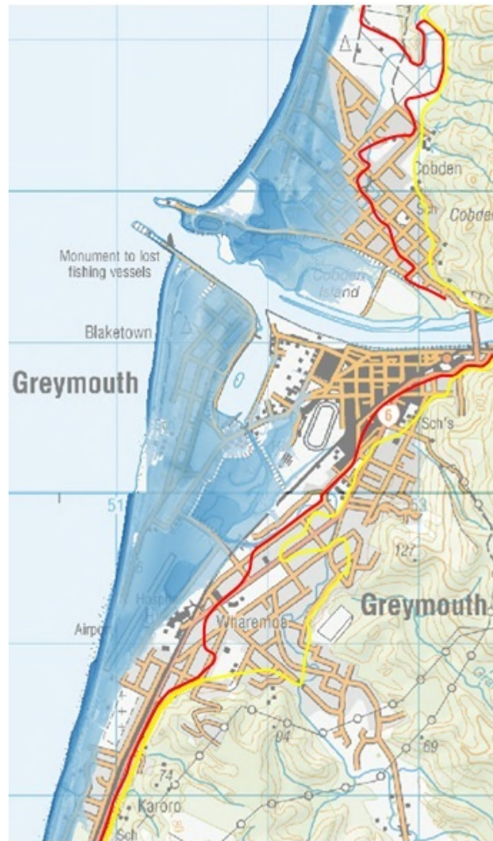
Figure 3.2: Greymouth - Estimated Inundation Area for 1:500 Tsunami Event
