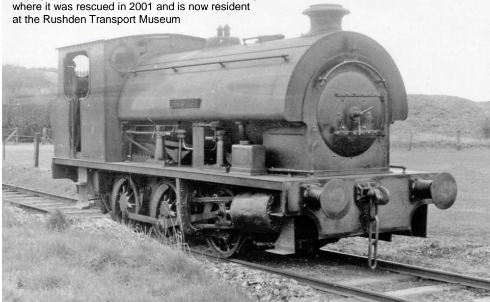
[2654] 0-6-0ST 'Cherwell' minus plates, undergoing some cosmetic painting Rushden Transport Museum, 15 th December 2012
