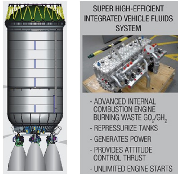
Figure 6. ACES concept with multiple engines and innovative IVF technology.
